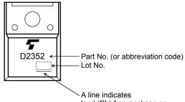
A line indicates lead (Pb)-free package or lead (Pb)-free finish.
