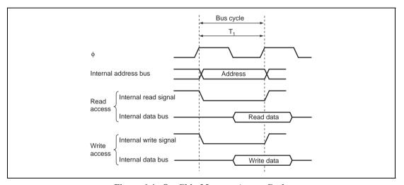
Figure 6.4 On-Chip Memory Access Cycle
