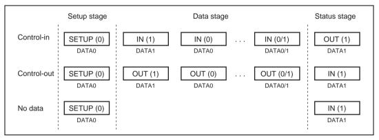
Figure 14.11 Control Transfer Stage Configuration
