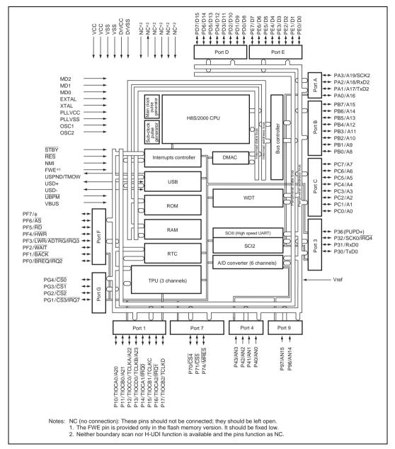
Figure 1.2 Internal Block Diagram of HD6432217
