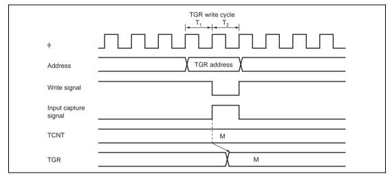
Figure 9.50 Contention between TGR Write and Input Capture
