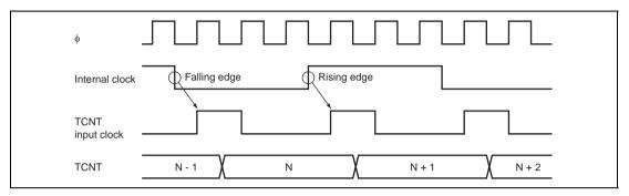
Figure 9.30 Count Timing in Internal Clock Operation
