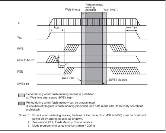
Figure 17.17 Power-On/Off Timing (User Program Mode)
