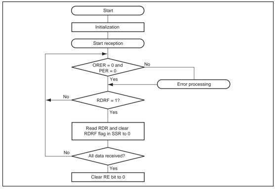
Figure 12.33 Example of Reception Processing Flow
