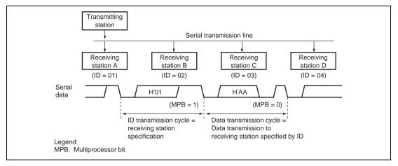
Figure 12.13 Example of Communication Using Multiprocessor Format (Transmission of Data H'AA to Receiving Station A)
