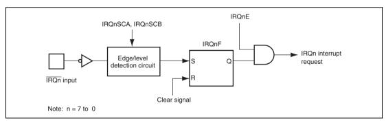
Figure 5.2 Block Diagram of Interrupts IRQn
