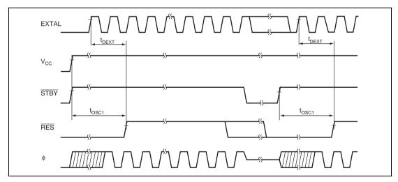
Figure 22.4 Oscillation Stabilization Timing
