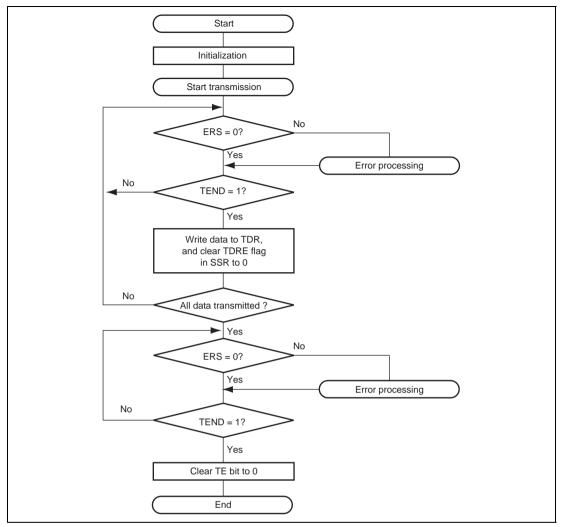
Figure 12.31 Example of Transmission Processing Flow
