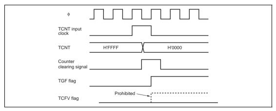
Figure 9.52 Contention between Overflow and Counter Clearing
