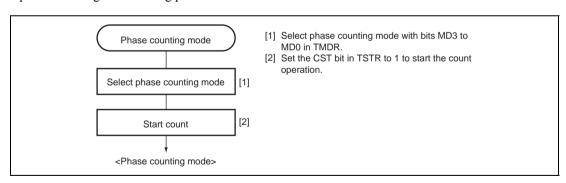
Figure 9.25 Example of Phase Counting Mode Setting Procedure
