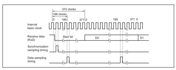
Figure 12.28 Receive Data Sampling Timing in Smart Card Mode (Using Clock of 372 Times the Transfer Rate)
