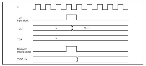
Figure 9.32 Output Compare Output Timing
