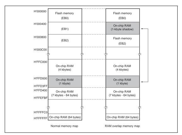
Figure 17.12 Example of RAM Overlap Operation
