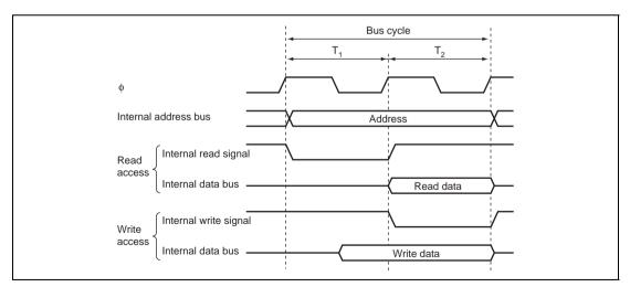
Figure 6.6 On-Chip Peripheral Module Access Cycle
