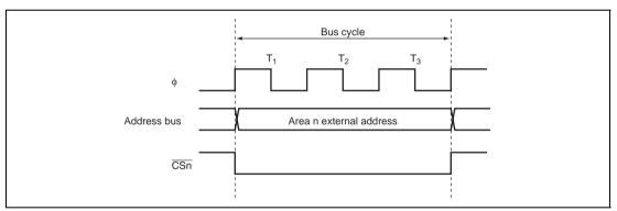
Figure 6.3  $\overline{CSn}$  Signal Output Timing (n = 0 to 5)
