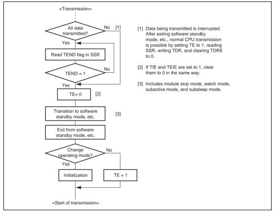
Figure 12.39 Sample Flowchart for Mode Transition during Transmission
