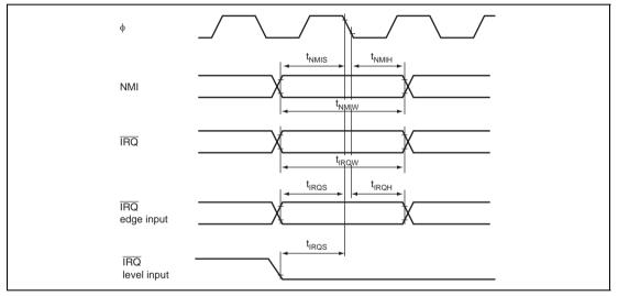
Figure 22.6 Interrupt Input Timing
