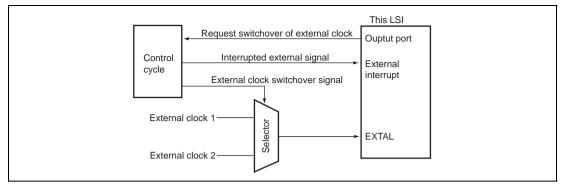
Figure 19.11 Example of External Clock Switching Circuit
