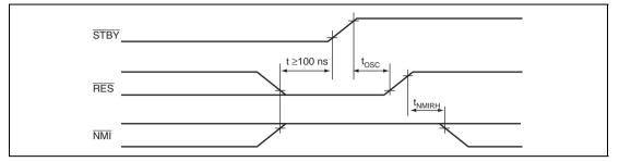
Figure 20.7 Timing of Recovery from Hardware Standby Mode
