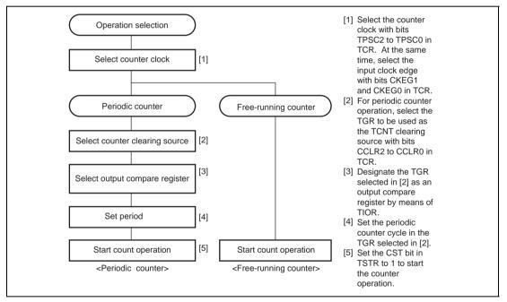
Figure 9.6 Example of Counter Operation Setting Procedure
