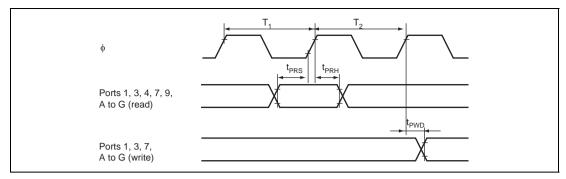
Figure 22.12 I/O Port Input/Output Timing
