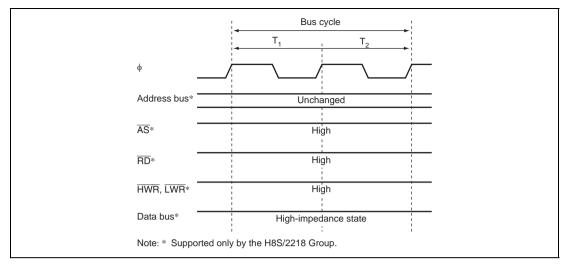
Figure 6.7 Pin States during On-Chip Peripheral Module Access
