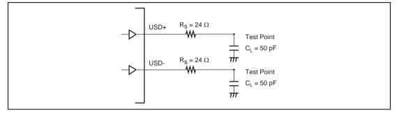
Figure 22.22 Test Load Circuit
