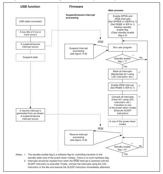
Figure 14.7 Example Flowchart of Suspend and Resume Operations
