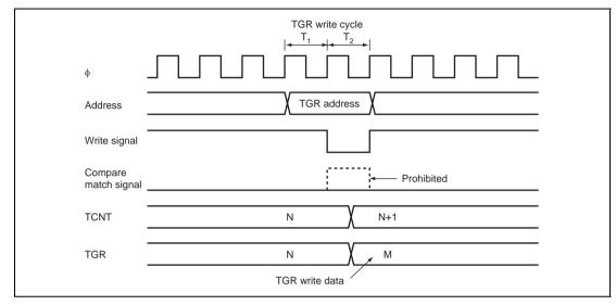
Figure 9.47 Contention between TGR Write and Compare Match
