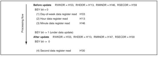
Figure 11.4 Example: Reading of Inaccurate Time Data
