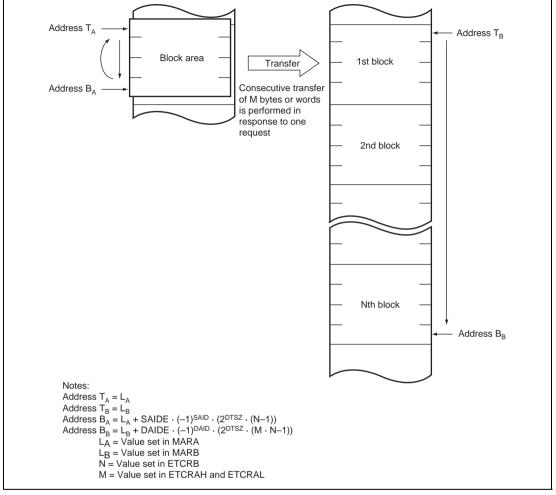
Figure 7.11 Operation in Block Transfer Mode (BLKDIR = 1)
