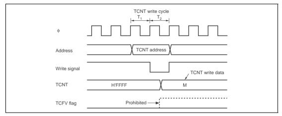
Figure 9.53 Contention between TCNT Write and Overflow
