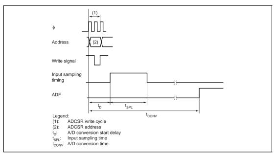
Figure 15.5 A/D Conversion Timing
