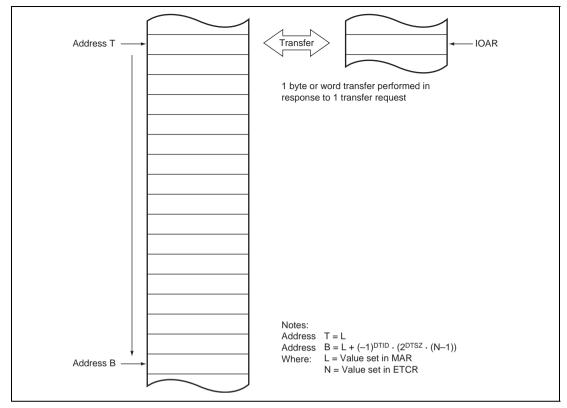
Figure 7.2 Operation in Sequential Mode
