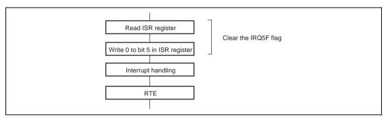
Figure 11.6 Example of RTC Interrupt Handling Routine
