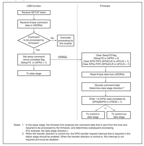
Figure 14.12 Setup Stage Operation
