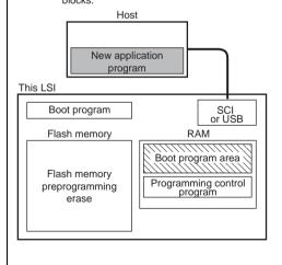
2. Programming control program transfer When boot mode is entered, the boot program in this LSI (originally incorporated in the chip) is started and the programming control program in the host is transferred to RAM via SCI or USB communication. The boot program required for flash memory erasing is automatically transferred to the RAM boot program area.
