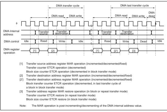
Figure 7.25 DMAC Register Update Timing
