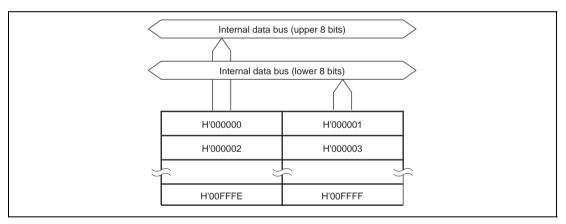
Figure 18.1 Block Diagram of On-Chip Masked ROM (64 kbytes)
