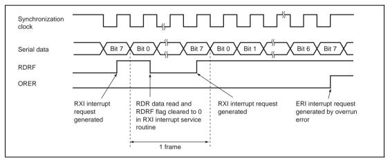
Figure 12.21 Example of SCI Operation in Reception
