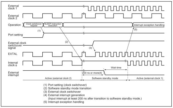
Figure 19.12 Example of External Clock Switchover Timing
