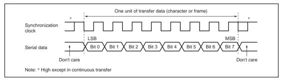
Figure 12.17 Data Format in Synchronous Communication (For LSB-First)
