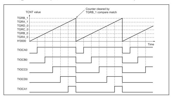
Figure 9.23 Example of PWM Mode Operation (2)
