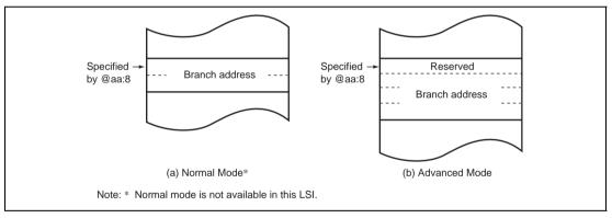
Figure 2.12 Branch Address Specification in Memory Indirect Mode
