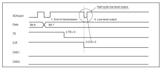
Figure 12.43 Operation when Switching from SCK Pin Function to Port Pin Function
