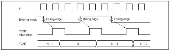
Figure 9.31 Count Timing in External Clock Operation
