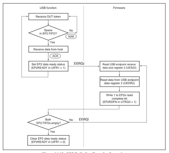
Figure 14.19 EP2 Bulk-Out Transfer Operation
