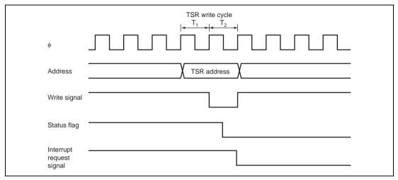
Figure 9.42 Timing for Status Flag Clearing by CPU
