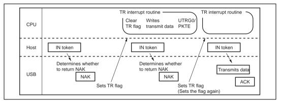
Figure 14.30 TR Interrupt Flag Set Timing
