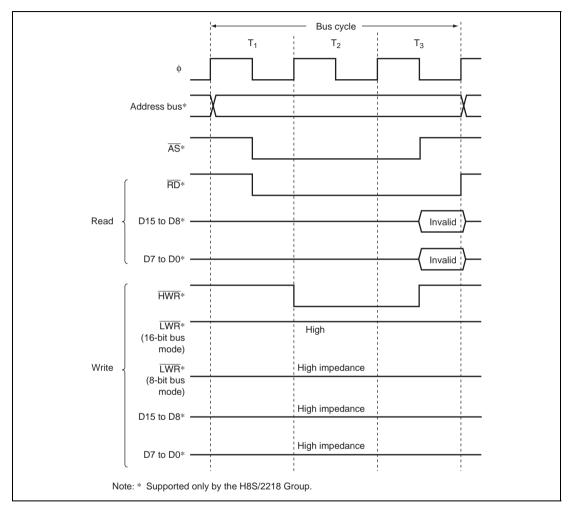
Figure 6.12 Bus Timing for Area 6 and RTC
