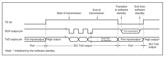
Figure 12.41 Port Pin State of Synchronous Transmission Using Internal Clock
