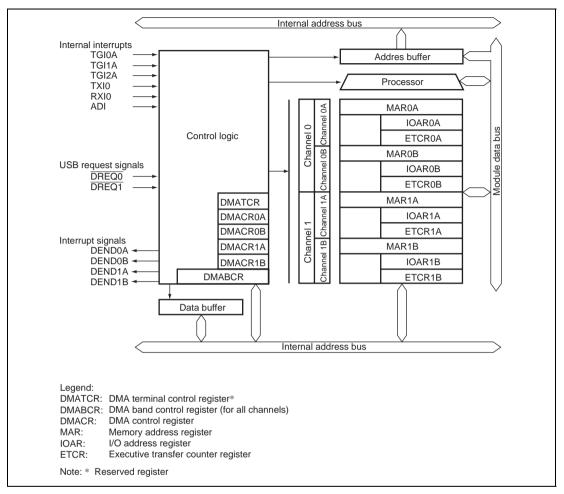
Figure 7.1 Block Diagram of DMAC
