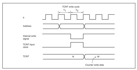
Figure 10.8 Contention between TCNT Write and Increment
