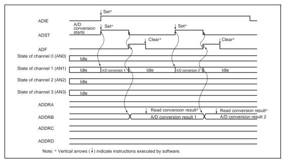
Figure 15.3 A/D Conversion Timing (Single-Chip Mode, Channel 1 Selected)
