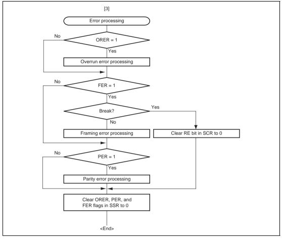
Figure 12.12 Sample Serial Data Reception Flowchart (2)
