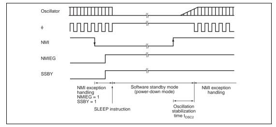
Figure 20.4 Software Standby Mode Application Example
