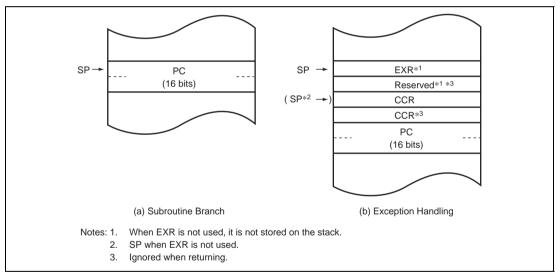
Figure 2.2 Stack Structure in Normal Mode
