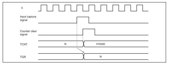
Figure 9.35 Counter Clear Timing (Input Capture)
