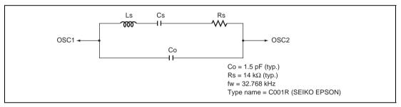
Figure 19.7 Equivalence Circuit for 32.768-kHz Oscillator
