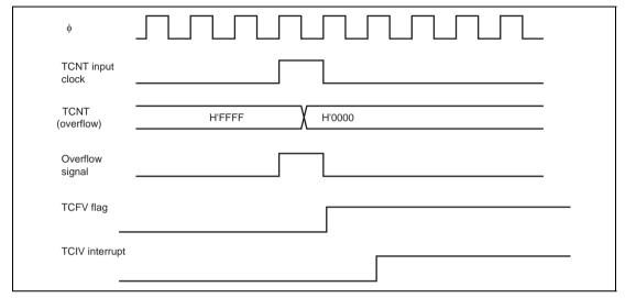
Figure 9.40 TCIV Interrupt Setting Timing
