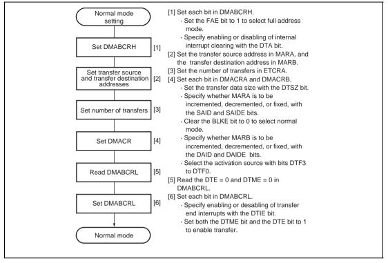
Figure 7.9 Example of Normal Mode Setting Procedure
