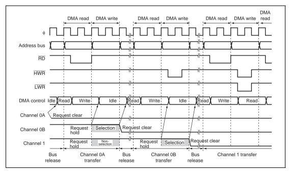
Figure 7.20 Example of Multi-Channel Transfer
