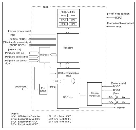
Figure 14.1 Block Diagram of USB
