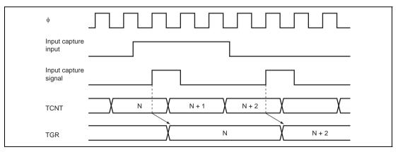
Figure 9.33 Input Capture Input Signal Timing
