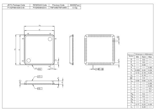
Figure C.4 TNP-64B and TNP-64BV Package Dimensions
