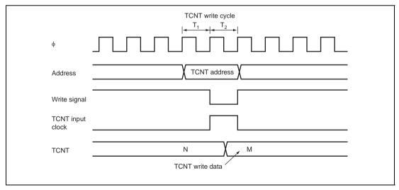
Figure 9.46 Contention between TCNT Write and Increment Operations
