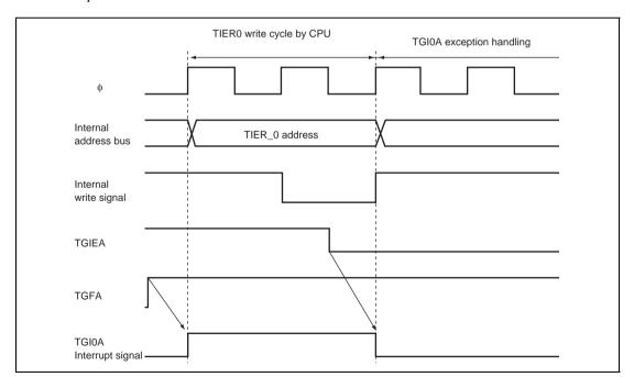
Figure 5.8 Contention between Interrupt Generation and Disabling
