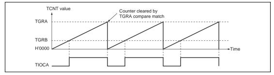
Figure 9.22 Example of PWM Mode Operation (1)
