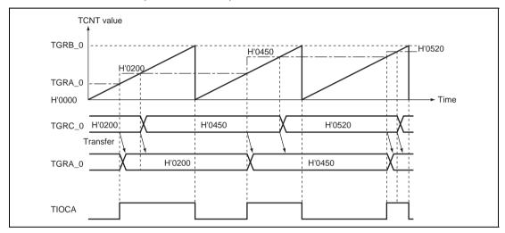
Figure 9.19 Example of Buffer Operation (1)
