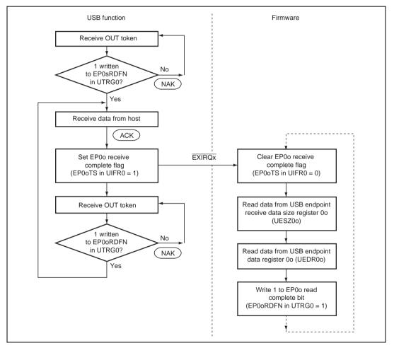
Figure 14.14 Data Stage Operation (Control-Out)
