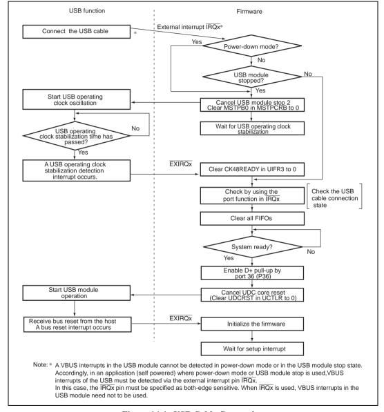
Figure 14.4 USB Cable Connection (When USB Module Stop or Power-Down Mode Is Used)
