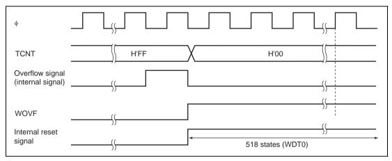
Figure 10.3 Timing of WOVF Setting
