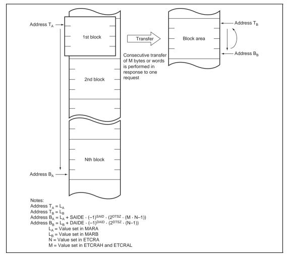
Figure 7.10 Operation in Block Transfer Mode (BLKDIR = 0)
