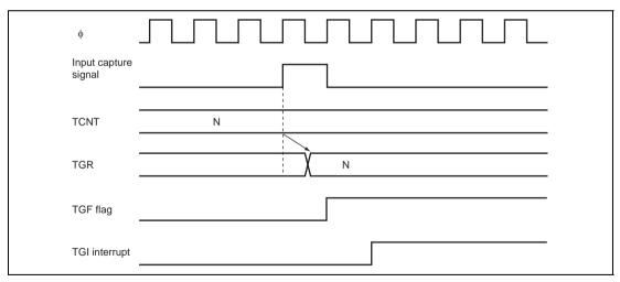
Figure 9.39 TGI Interrupt Timing (Input Capture)
