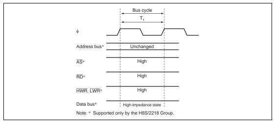
Figure 6.5 Pin States during On-Chip Memory Access
