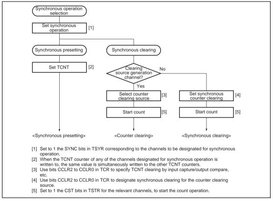
Figure 9.14 Example of Synchronous Operation Setting Procedure
