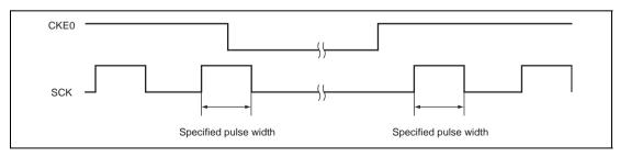
Figure 12.34 Timing for Fixing Clock Output Level
