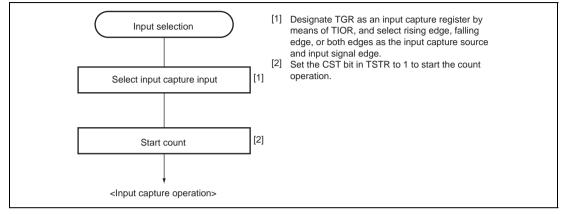
Figure 9.12 Example of Input Capture Operation Setting Procedure
