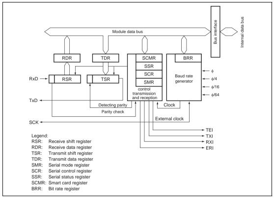
Figure 12.2 Block Diagram of SCI 2
