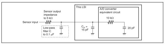
Figure 15.9 Example of Analog Input Circuit
