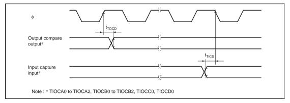
Figure 22.13 TPU Input/Output Timing
