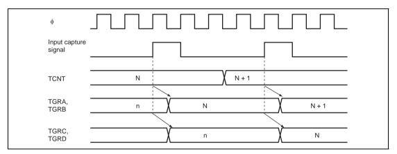
Figure 9.37 Buffer Operation Timing (Input Capture)
