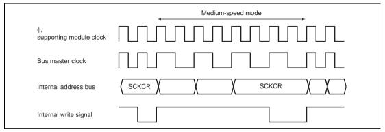
Figure 20.3 Medium-Speed Mode Transition and Clearance Timing
