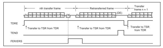
Figure 12.29 Retransfer Operation in SCI Transmit Mode
