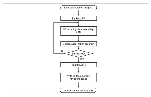
Figure 17.11 Flowchart for Flash Memory Emulation in RAM
