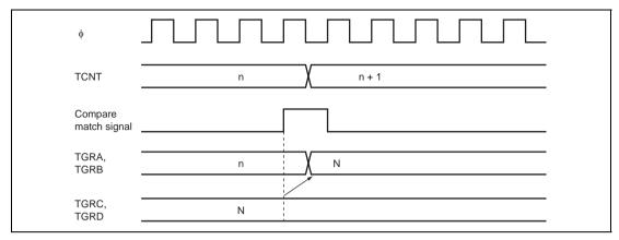
Figure 9.36 Buffer Operation Timing (Compare Match)
