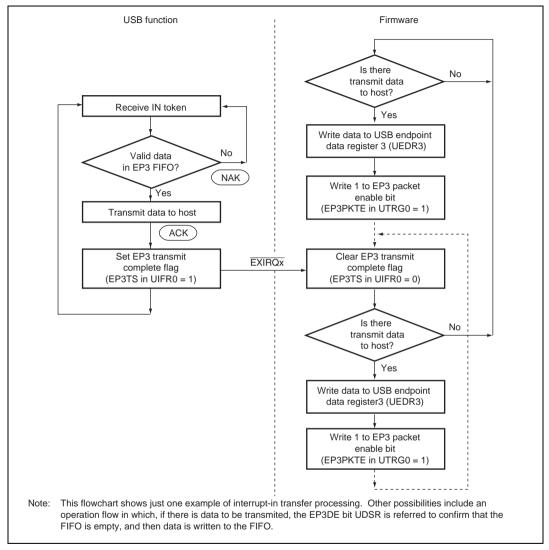
Figure 14.17 EP3 Interrupt-In Transfer Operation
