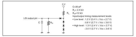
Figure 22.2 Output Load Circuit
