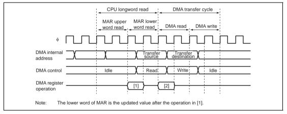
Figure 7.26 Contention between DMAC Register Update and CPU Read
