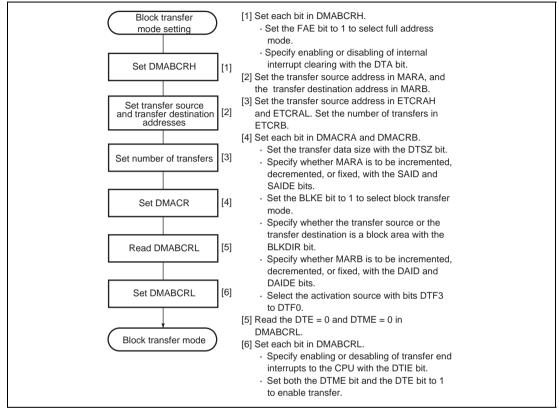
Figure 7.13 Example of Block Transfer Mode Setting Procedure
