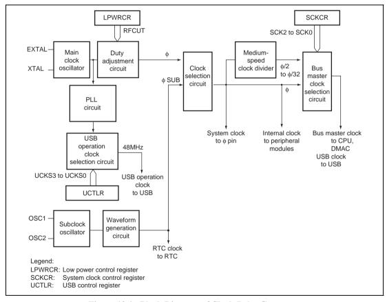
Figure 19.1 Block Diagram of Clock Pulse Generator
