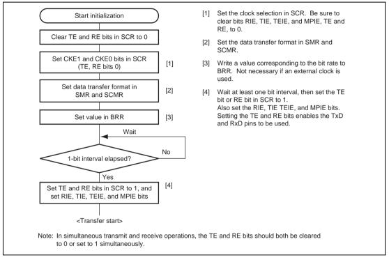
Figure 12.18 Sample SCI Initialization Flowchart
