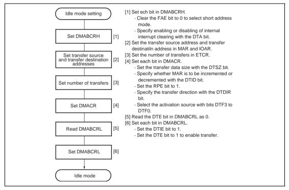
Figure 7.5 Example of Idle Mode Setting Procedure
