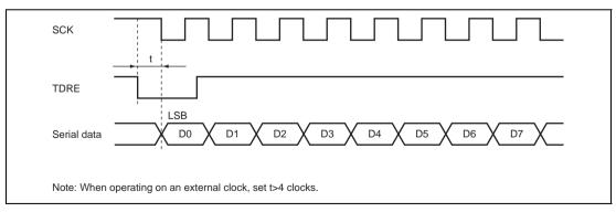
Figure 12.38 Example of Clocked Synchronous Transmission by DMAC
