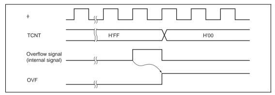
Figure 10.5 Timing of OVF Setting
