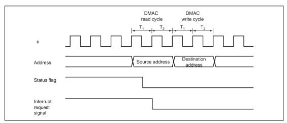
Figure 9.43 Timing for Status Flag Clearing by DMAC Activation
