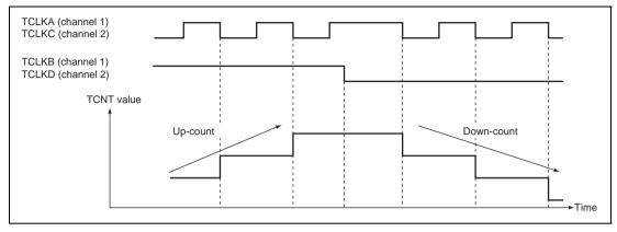
Figure 9.27 Example of Phase Counting Mode 2 Operation
