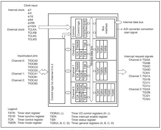
Figure 9.1 Block Diagram of TPU
