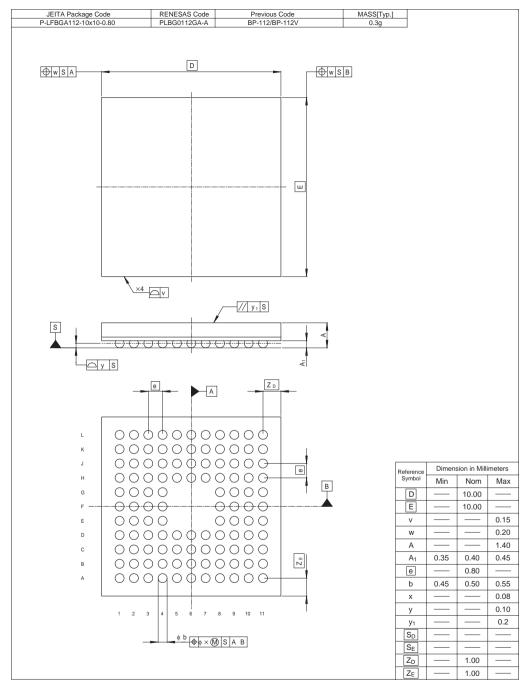
Figure C.2 BP-112 and BP-112V Package Dimensions
