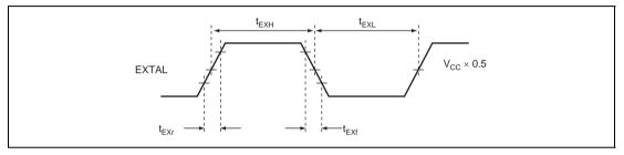
Figure 19.5 External Clock Input Timing
