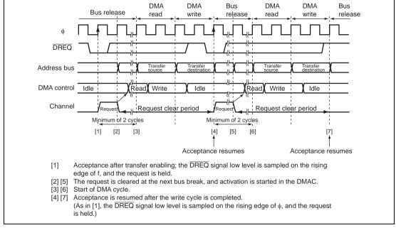
Figure 7.19 Example of DREQ Level Activated Normal Mode Transfer
