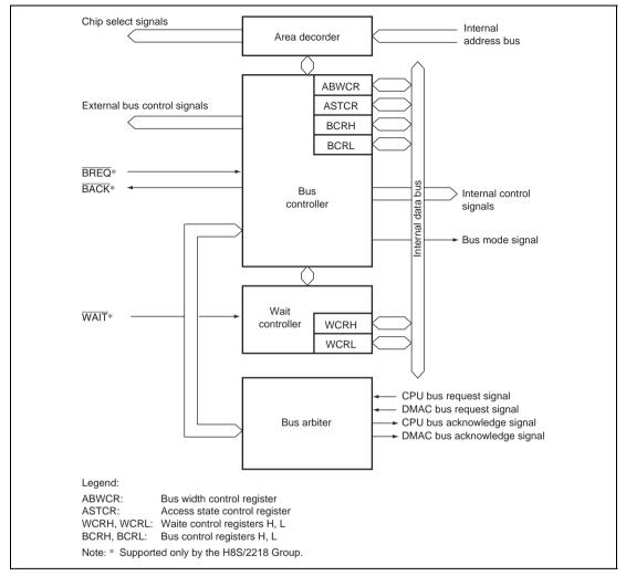
Figure 6.1 Block Diagram of Bus Controller
