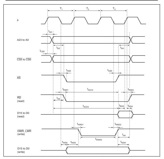
Figure 22.8 Basic Bus Timing (Three-State Access)
