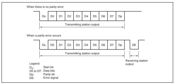
Figure 12.25 Normal Smart Card Interface Data Format
