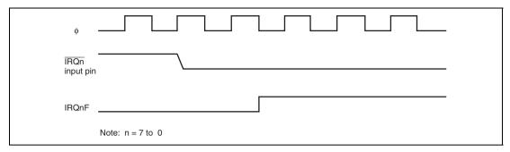
Figure 5.3 Timing of Setting IRQnF
