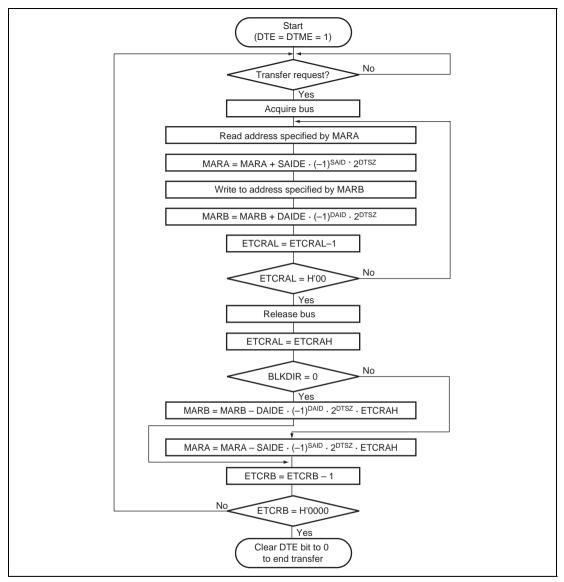
Figure 7.12 Operation Flow in Block Transfer Mode
