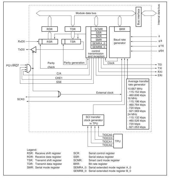
Figure 12.1 Block Diagram of SCI\_0
