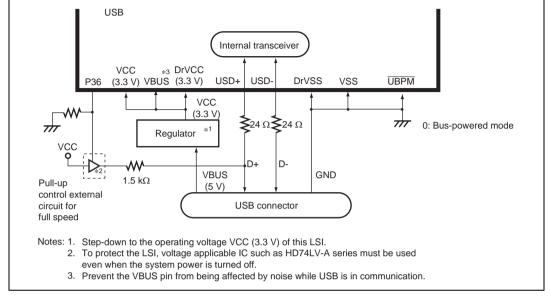
Figure 14.26 USB External Circuit in Bus-Powered Mode
