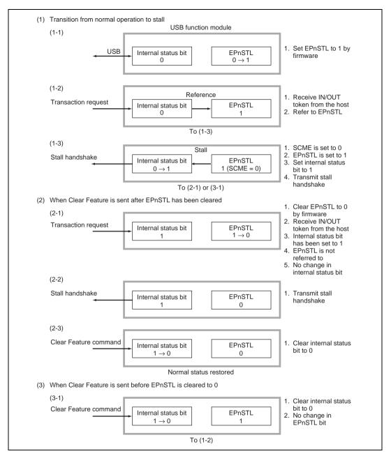
Figure 14.20 Forcible Stall by Firmware
