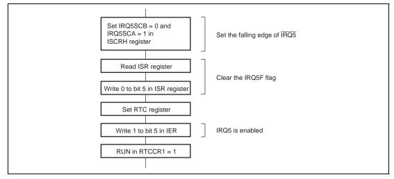
Figure 11.5 Initializing Procedure in Using RTC Interrupt
