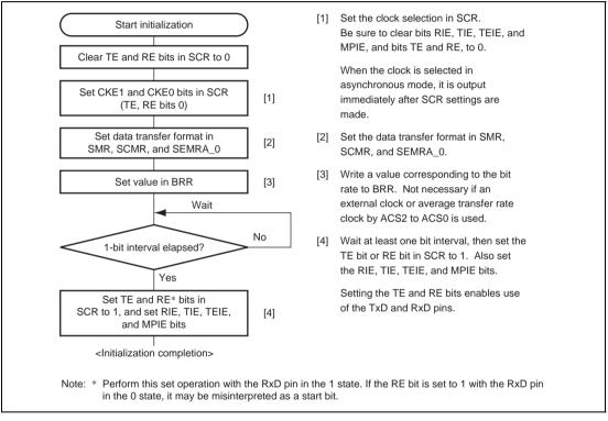
Figure 12.8 Sample SCI Initialization Flowchart
