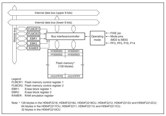
Figure 17.1 Block Diagram of Flash Memory
