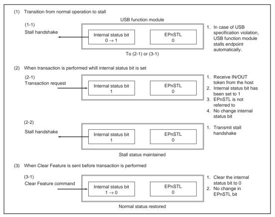
Figure 14.21 Automatic Stall by USB Function Module
