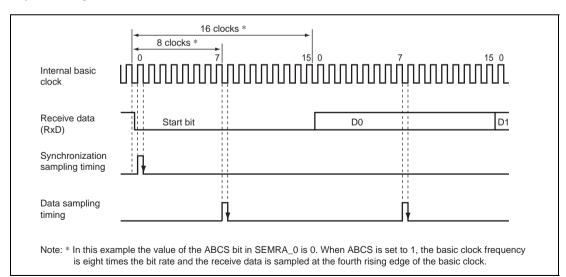
Figure 12.6 Receive Data Sampling Timing in Asynchronous Mode
