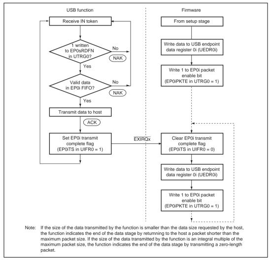
Figure 14.13 Data Stage Operation (Control-In)
