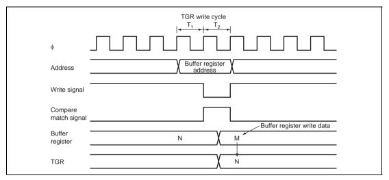
Figure 9.48 Contention between Buffer Register Write and Compare Match
