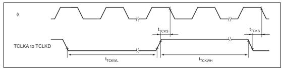
Figure 22.14 TPU Clock Input Timing
