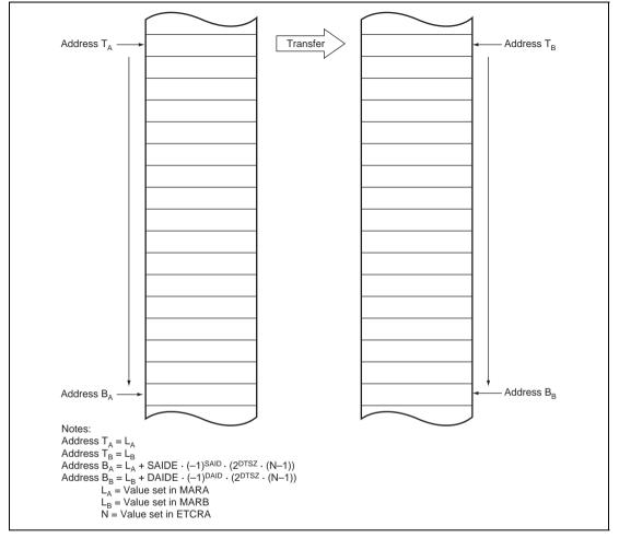
Figure 7.8 Operation in Normal Mode
