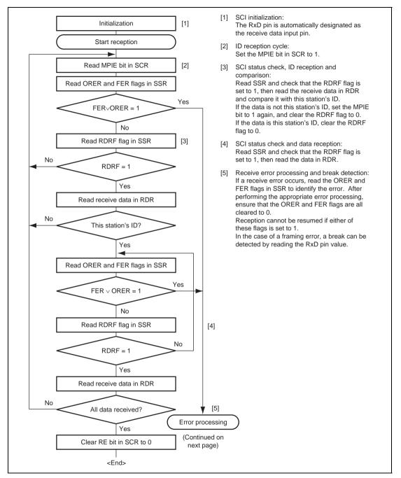
Figure 12.16 Sample Multiprocessor Serial Data Reception Flowchart (1)
