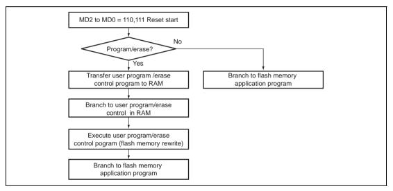
Figure 17.10 Programming/Erasing Flowchart Example in User Program Mode
