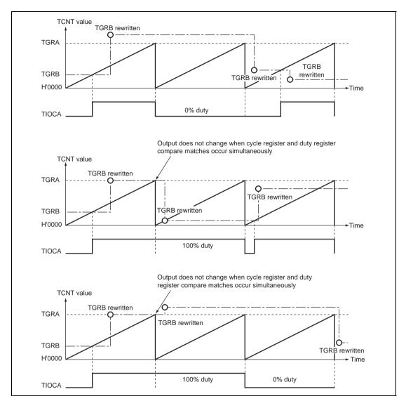
Figure 9.24 Example of PWM Mode Operation (3)
