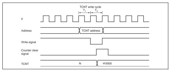
Figure 9.45 Contention between TCNT Write and Clear Operations
