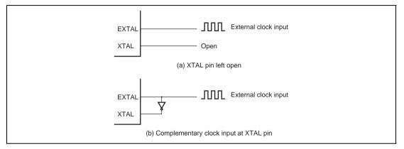
Figure 19.4 External Clock Input (Examples)
