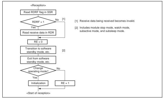
Figure 12.42 Sample Flowchart for Mode Transition during Reception
