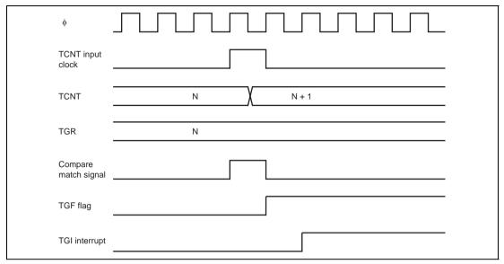
Figure 9.38 TGI Interrupt Timing (Compare Match)
