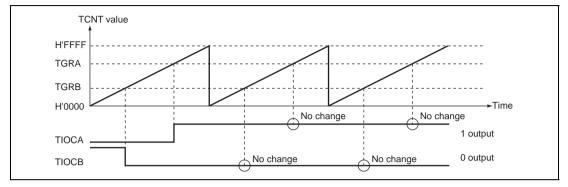
Figure 9.10 Example of 0 Output/1 Output Operation
