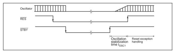
Figure 20.5 Hardware Standby Mode Timing (Example)
