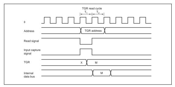
Figure 9.49 Contention between TGR Read and Input Capture
