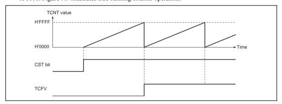
Figure 9.7 Free-Running Counter Operation
