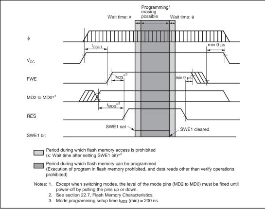
Figure 17.16 Power-On/Off Timing (Boot Mode)
