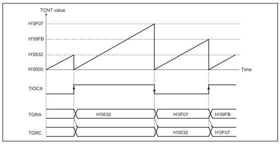
Figure 9.20 Example of Buffer Operation (2)
