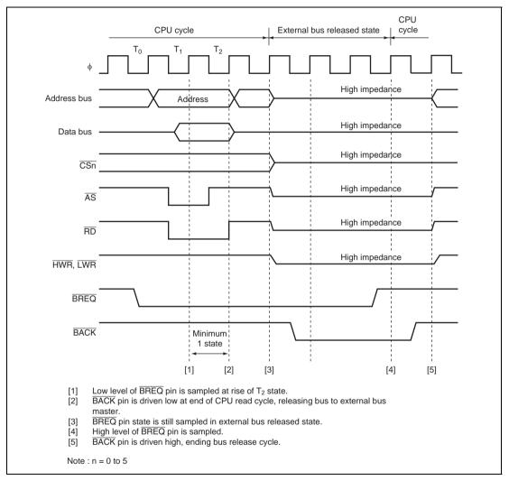
Figure 6.25 Bus-Released State Transition Timing
