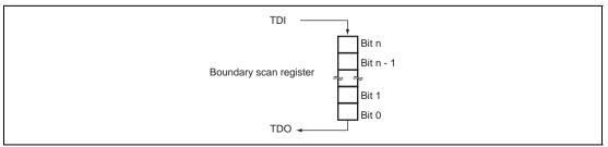
Figure 13.5 Serial Data Input/Output
