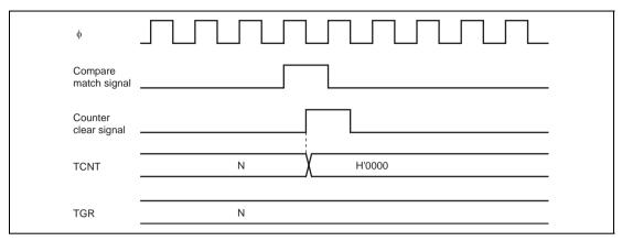
Figure 9.34 Counter Clear Timing (Compare Match)
