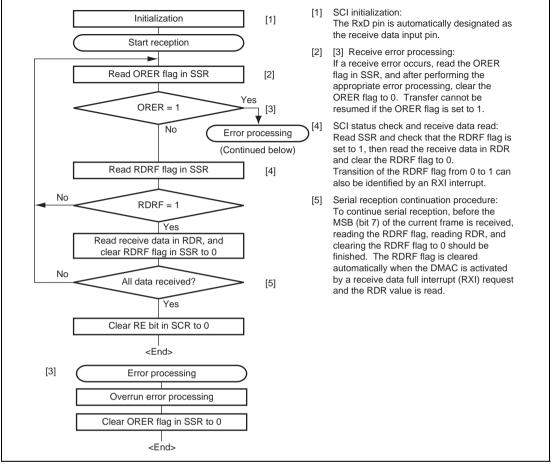
Figure 12.22 Sample Serial Data Reception Flowchart
