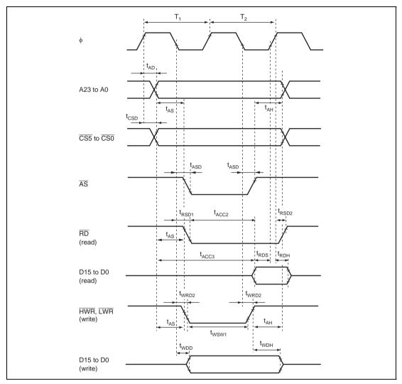
Figure 22.7 Basic Bus Timing (Two-State Access)
