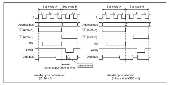
Figure 6.23 Example of Idle Cycle Operation (2)
