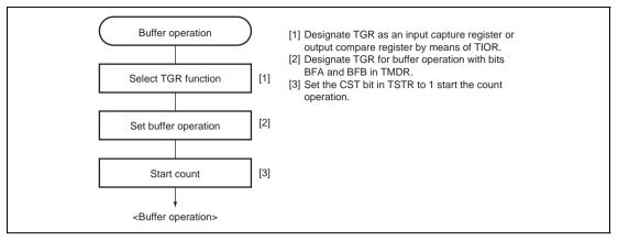
Figure 9.18 Example of Buffer Operation Setting Procedure
