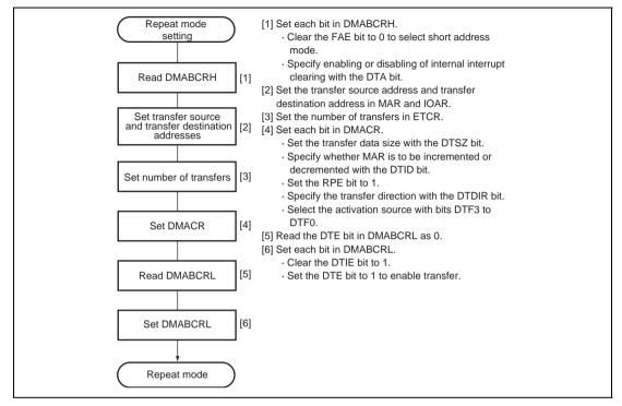
Figure 7.7 Example of Repeat Mode Setting Procedure
