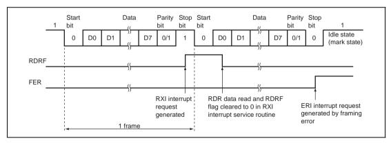
Figure 12.11 Example of SCI Operation in Reception (Example with 8-Bit Data, Parity, One Stop Bit)
