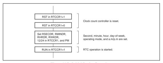
Figure 11.3 Initial Setting Procedure
