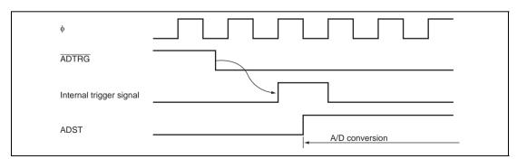
Figure 15.6 External Trigger Input Timing
