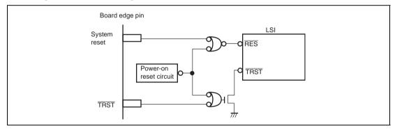
Figure 13.4 Recommended Reset Signal Design
