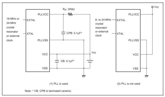
Figure 19.9 Example of PLL Circuit
