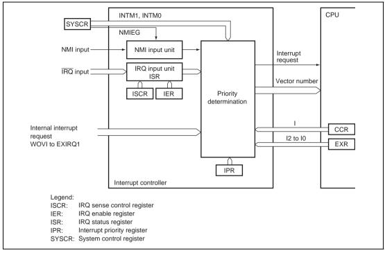
Figure 5.1 Block Diagram of Interrupt Controller
