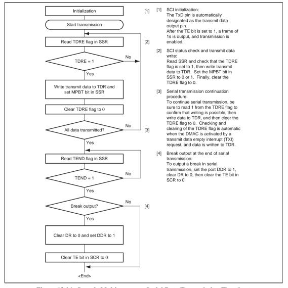
Figure 12.14 Sample Multiprocessor Serial Data Transmission Flowchart
