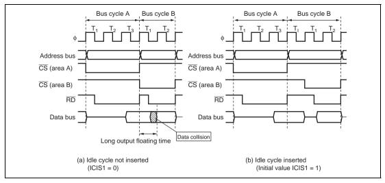
Figure 6.22 Example of Idle Cycle Operation (1)
