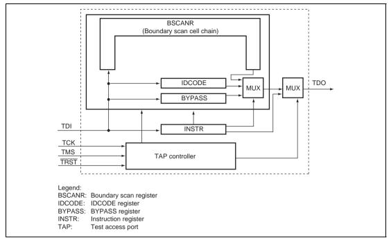
Figure 13.1 Block Diagram of Boundary Scan Function
