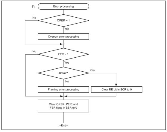
Figure 12.16 Sample Multiprocessor Serial Data Reception Flowchart (2)
