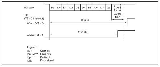
Figure 12.30 TEND Flag Generation Timing in Transmission Operation
