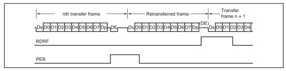
Figure 12.32 Retransfer Operation in SCI Receive Mode
