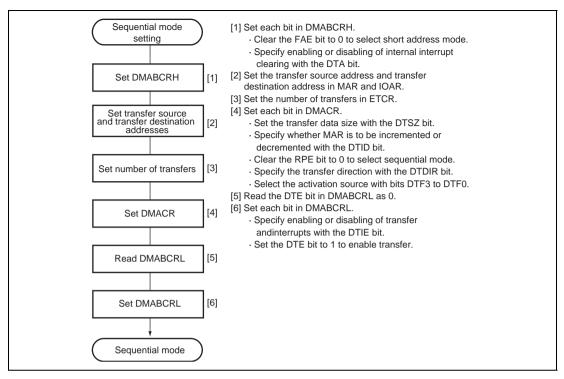
Figure 7.3 Example of Sequential Mode Setting Procedure
