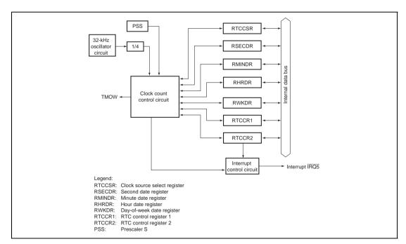
Figure 11.1 Block Diagram of RTC
