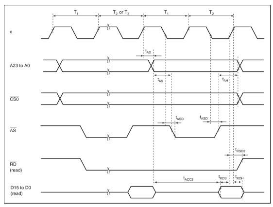
Figure 22.10 Burst ROM Access Timing (Two-State Access)
