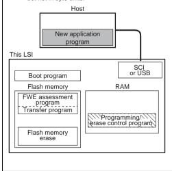
Programming/erase control program transfer When user program mode is entered, user software confirms this fact, executes transfer program in the flash memory, and transfers the programming/erase control program to RAM.
