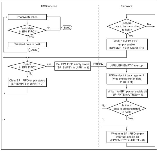
Figure 14.18 EP1 Bulk-In Transfer Operation
