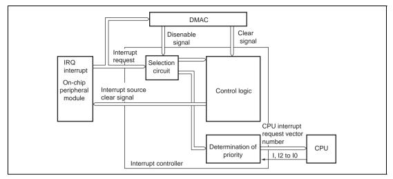
Figure 5.7 Interrupt Control for DMAC
