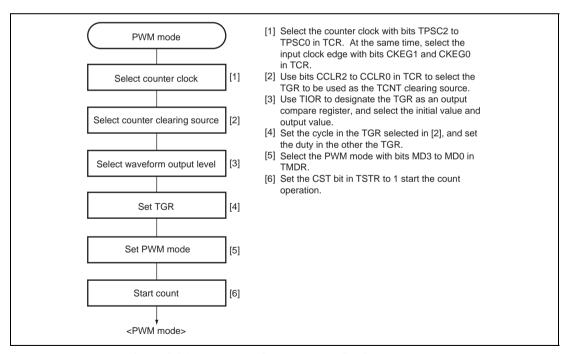
Figure 9.21 Example of PWM Mode Setting Procedure
