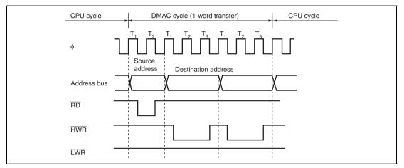
Figure 7.14 Example of DMA Transfer Bus Timing
