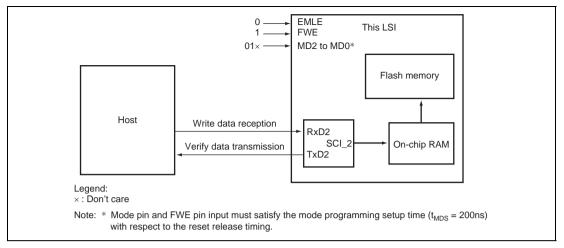
Figure 17.8 System Configuration in SCI Boot Mode
