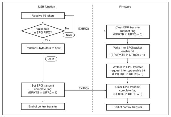
Figure 14.16 Status Stage Operation (Control-Out)
