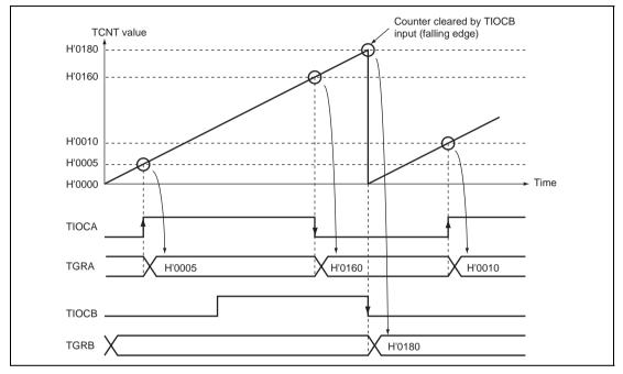
Figure 9.13 Example of Input Capture Operation
