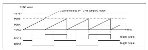
Figure 9.11 Example of Toggle Output Operation
