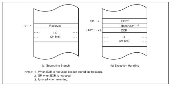
Figure 2.4 Stack Structure in Advanced Mode
