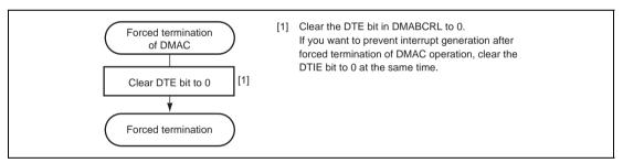
Figure 7.22 Example of Procedure for Forcibly Terminating DMAC Operation
