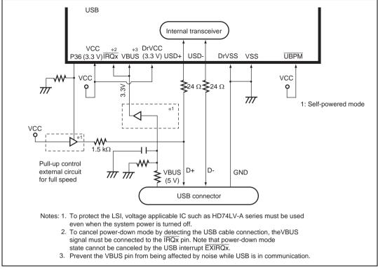
Figure 14.27 USB External Circuit in Self-Powered Mode
