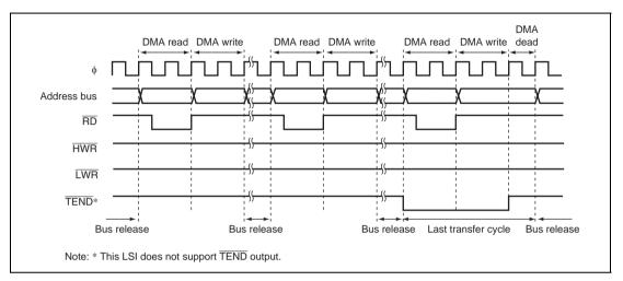
Figure 7.15 Example of Short Address Mode Transfer
