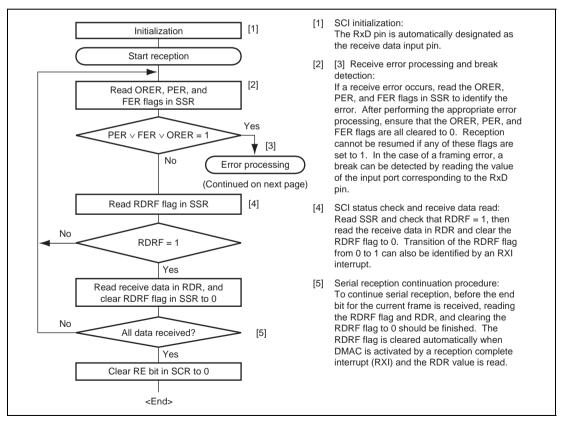
Figure 12.12 Sample Serial Data Reception Flowchart (1)
