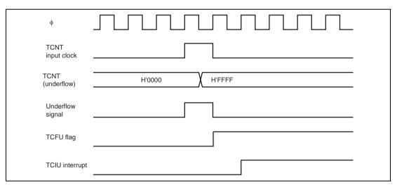
Figure 9.41 TCIU Interrupt Setting Timing
