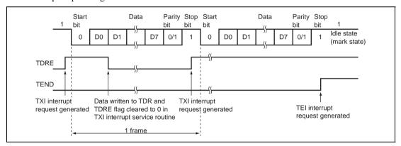
Figure 12.9 Example of Operation in Transmission in Asynchronous Mode (Example with 8-Bit Data, Parity, One Stop Bit)
