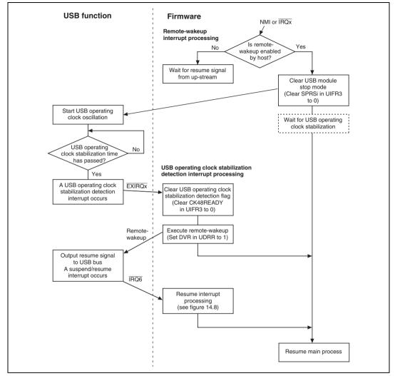
Figure 14.10 Example Flowchart of Remote-Wakeup Interrupt Processing
