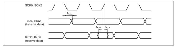
Figure 22.16 SCI Input/Output Timing (Clock Synchronous Mode)
