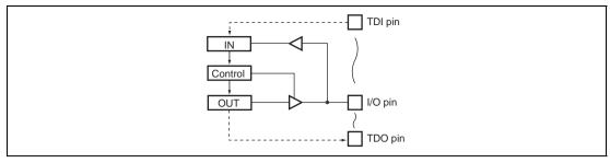
Figure 13.2 Boundary Scan Register Configuration
