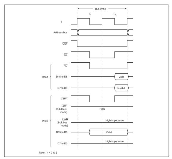
Figure 6.10 Bus Timing for 8-Bit 2-State Access Space
