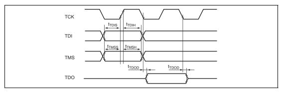
Figure 22.20 Boundary Scan Data Transmission Timing
