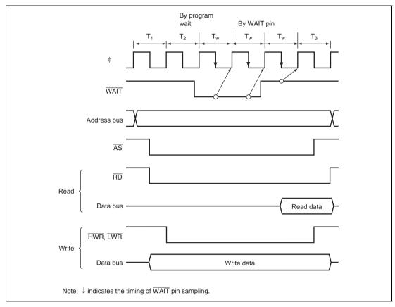
Figure 6.19 Example of Wait State Insertion Timing
