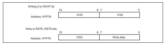
Figure 10.7 Format of Data Written to RSTCSR (Example of WDT0)
