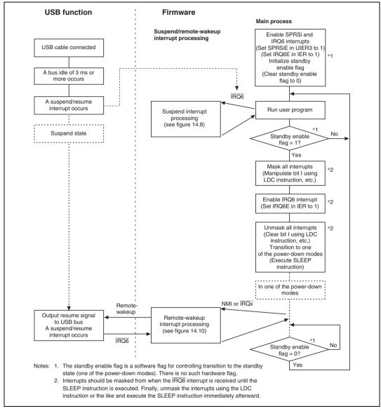
Figure 14.9 Example Flowchart of Suspend and Remote-Wakeup Operations
