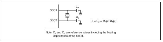
Figure 19.6 Example Connection of 32.768-kHz Quartz Oscillator
