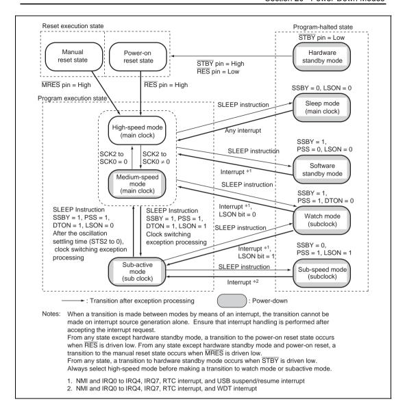
Figure 20.1 Mode Transition Diagram
