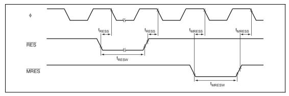
Figure 22.5 Reset Input Timing
