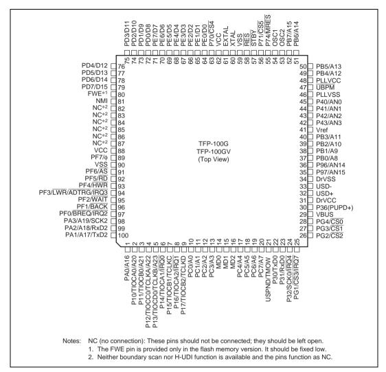
Figure 1.7 Pin Arrangements of HD6432217 (TFP-100G, TFP-100GV)
