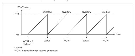
Figure 10.4 Operation in Interval Timer Mode
