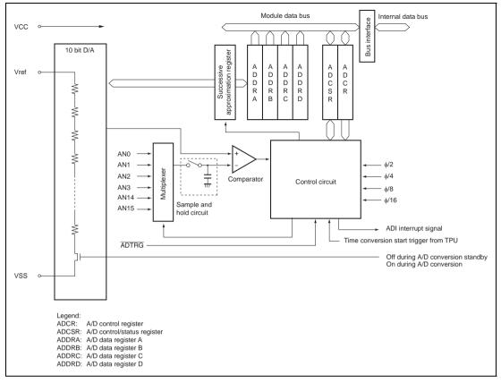
Figure 15.1 Block Diagram of A/D Converter
