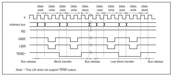
Figure 7.18 Example of Full Address Mode (Block Transfer Mode) Transfer
