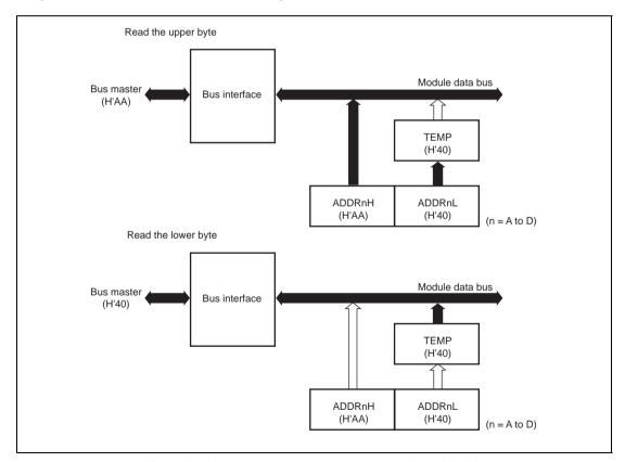
Figure 15.2 Access to ADDR (When Reading H'AA40)
