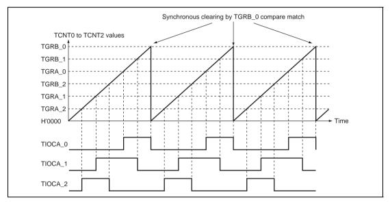
Figure 9.15 Example of Synchronous Operation
