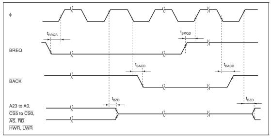
Figure 22.11 External Bus Release Timing
