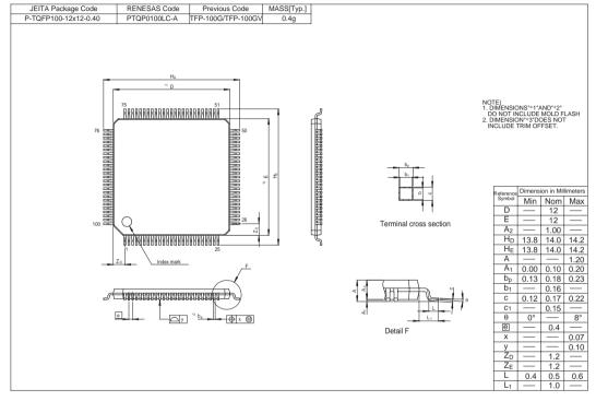
Figure C.1 TFP-100G and TFP-100GV Package Dimensions
