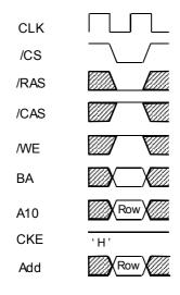
The EM488M3244VBA have 4 banks, each with 4,096 rows. This command activates the bank selected by BA and a row address selected by A0 through A11.This command corresponds to a conventional DRAM's /RAS falling.
