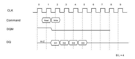
Read can be interrupted by Write. DQM must be high at least 3 clicks prior to the write command.
