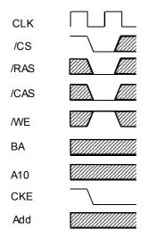
After the command execution, self refresh operation continues while CKE remains low. When CKE goes high, the memory exits the self refresh mode. During self refresh mode, refresh interval and refresh operation are performed internally, so there before is no need for external control. Before executing self refresh, both banks must be precharged.
