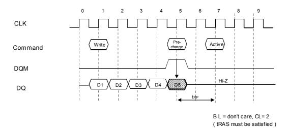
When /CAS Latency is 3, the write data written prior to the precharge command will be correctly stored. However, invalid data may be written at the same clock as the precharge command. In order to avoid this situation, DQM must be high at the same clock as the precharge command. This will mask the invalid data.
