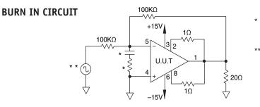
These components are used to stabilize device due to poor high frequency characteristics of burn in board.
