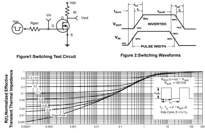
Square Wave Pluse Duration(sec) Figure 3: Normalized Maximum Transient Thermal Impedance
