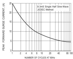
FIG.5 MAXIMUM NON-REPETITIVE FORWARD SURGE CURRENT
