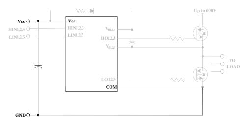
Figure 21: Supply capacitor
