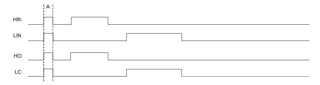
Figure 4: Input/output timing diagram
