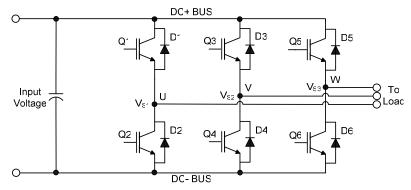
Figure 11: Three phase inverter
