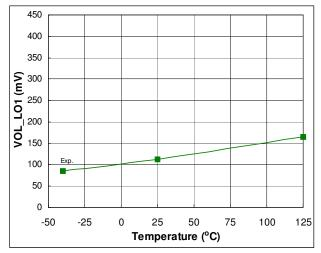
Fig. 29. Low Level Output Voltage vs. Temperature
