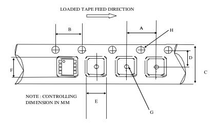
CARRIER TAPE DIMENSION FOR 8SOICN
