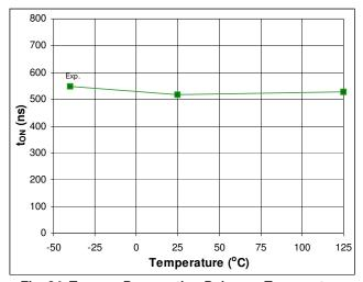
Fig. 24. Turn-on Propagation Delay vs. Temperature
