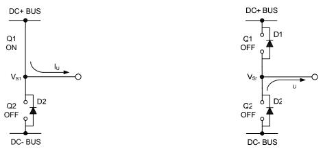
Figure 12: Q1 conducting
