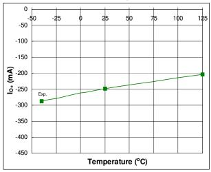
Fig. 39. Output High Short Circuit Pulsed Current vs. Temperature
