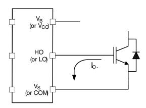
Figure 2: HVIC sinking current
