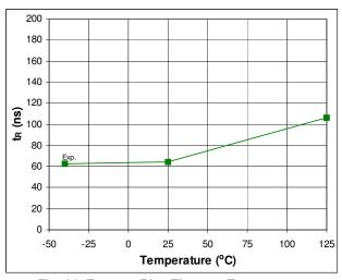
Fig. 26. Turn-on Rise Time vs. Temperature
