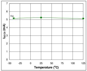
Fig. 32. Quiescent VCC Supply Current vs. Temperature
