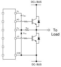
Figure 23: V<sub>S</sub> clamping diode
