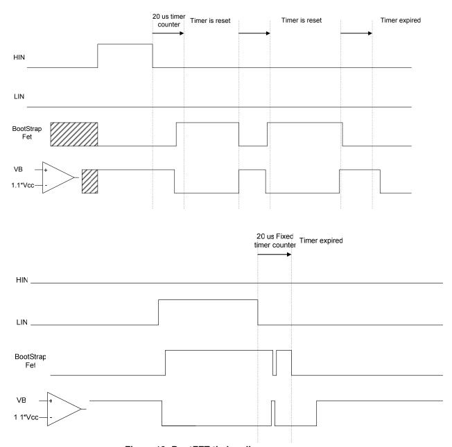
Figure 10: BootFET timing diagram
