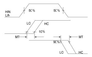
Figure 6: Delay Matching Waveform Definition
