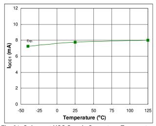
Fig. 31. Quiescent VCC Supply Current vs. Temperature
