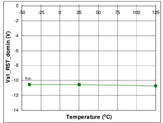
Fig. 41. Max -Vs vs. Temperature
