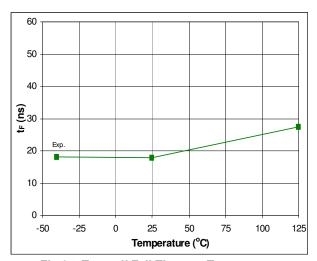
Fig.27. Turn-off Fall Time vs. Temperature
