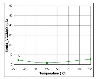
Fig. 30. Offset Supply Leakage Current vs. Temperature
