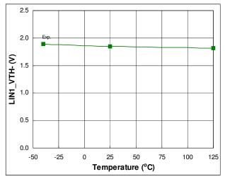
Fig. 28. Input Negative Going Threshold vs. Temperature
