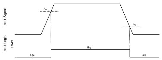
Figure 7: HIN & LIN input thresholds
