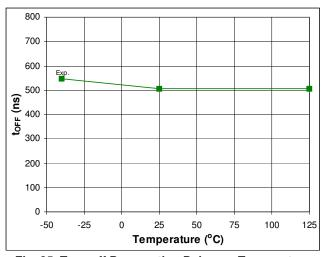
Fig. 25. Turn-off Propagation Delay vs. Temperature
