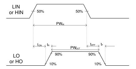
Figure 3: Switching time waveforms
