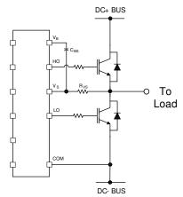
Figure 22: V<sub>S</sub> resistor
