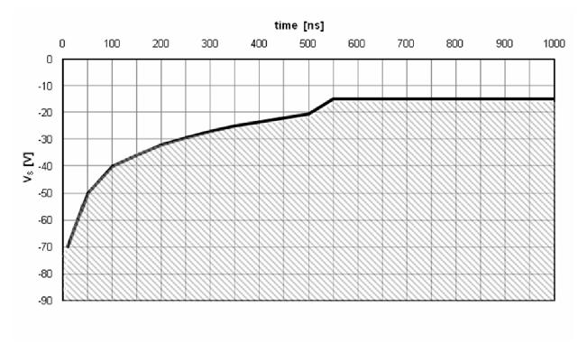
Figure 19: Negative V<sub>S</sub> transient SOA @ VBS=15V
