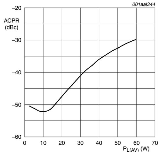
$V_{DS} = 28\text{ V}; I_{Dq} = 950\text{ mA}; f = 2140\text{ MHz};$
