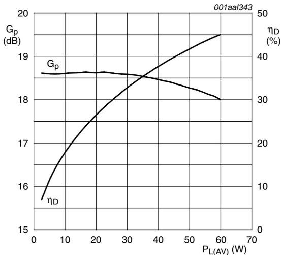
$V_{DS} = 28\text{ V}; I_{Dq} = 950\text{ mA}; f = 2140\text{ MHz}.$
