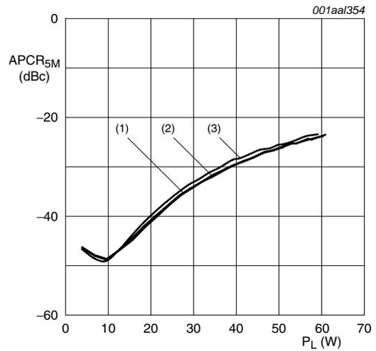
$V_{DS} = 28\text{ V}$ ;  $I_{Dq} = 950\text{ mA}$ ; carrier spacing 5 MHz.
