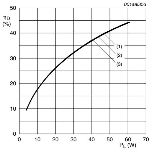
$V_{DS} = 28\text{ V}$ ;  $I_{Dq} = 950\text{ mA}$ ; carrier spacing 5 MHz.
