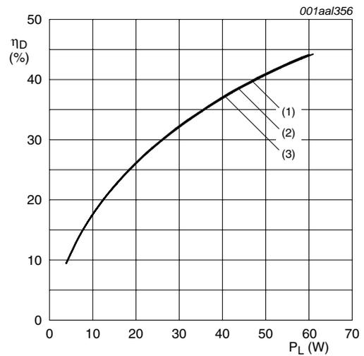
$V_{DS} = 28\text{ V}$ ;  $I_{Dq} = 950\text{ mA}$ ; carrier spacing 10 MHz.
