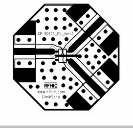
PCB material (FR4), PCB thickness (0.8t), Via hole ( $\phi$ 0.7)
