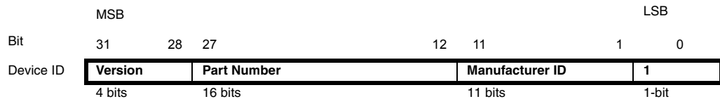
Figure 26-1. The Format of the Device Identification Register
