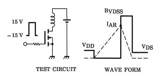
$$\begin{aligned} &R_G = 25~\Omega \\ &V_{DD} = 90~V,~L = 12.2~mH \end{aligned} \qquad E_{AS} = \frac{1}{2} \cdot L \cdot I^2 \cdot \left( \frac{B_{VDSS}}{B_{VDSS} - V_{DD}} \right)$$
