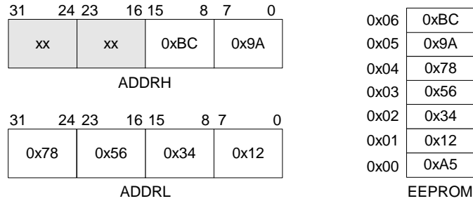
Figure 5.2 Example ADDR1, ADDR0 and EEPROM Setup
