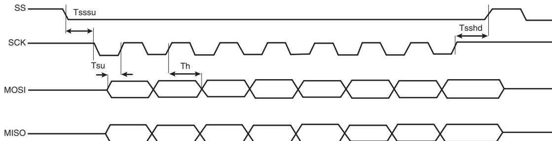
Figure 7-3. Read Status Register to Release IRQ
