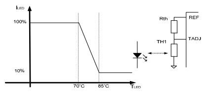
Thermal network response in Buck configuration with: Rth =  $2k\Omega$  and TH1= $10k\Omega$  (beta =3900)
