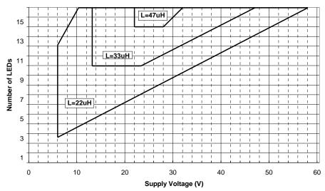
Figure 26: 350mA Buck-Boost mode inductor selection for target frequency > 500kHz Suitable coils for use with the ZXLD1370 may be selected from the MSS range manufactured by Coilcraft, or the NPIS range manufactured by NIC components.
