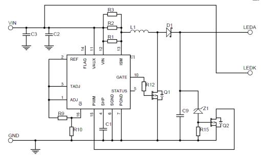
Figure 45: Application circuit - 700mA Buck-Boost LED driver
