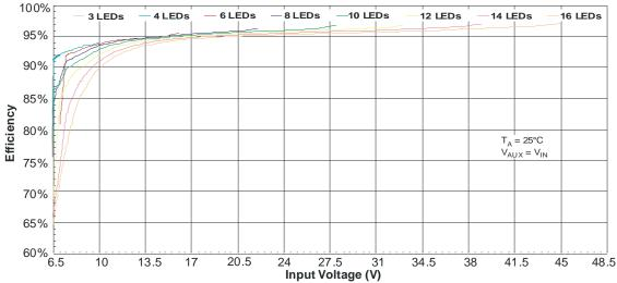
Figure 9: Efficiency vs. Input Voltage & Number of LED
