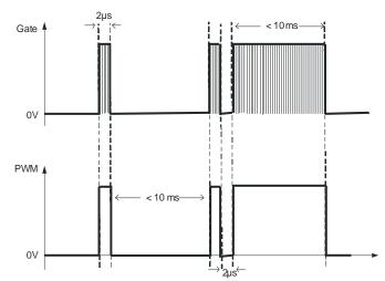
Figure 31:PWM dimming minimum and maximum pulse
