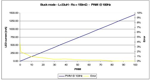
Figure 28: LED current linearity and accuracy with PWM dimming at 100Hz
