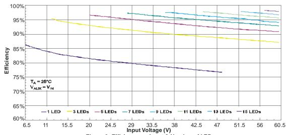
Figure 3: Efficiency vs. Input & Number of LED
