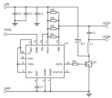
Figure 39: Application circuit: 2.8A Buck LED driver
