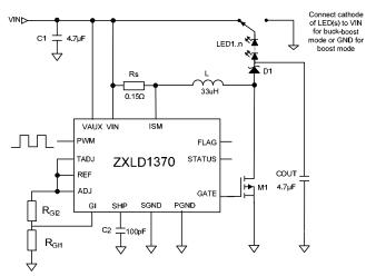
Figure 15: Boost and Buck-Boost configuration
