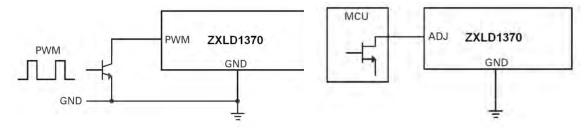
Figure 29: PWM dimming from open collector switch
