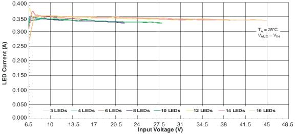
Figure 7: I<sub>LED</sub> vs. Input Voltage & Number of LED
