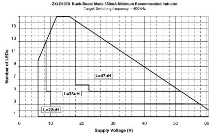
Figure 23: 350mA Buck-Boost mode inductor selection for target frequency 400kHz
