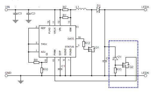
Fig 37: OVP circuit
