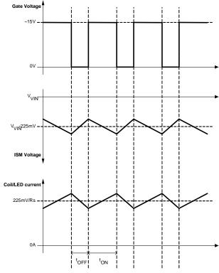
Figure 14: Operating waveforms (Buck mode)
