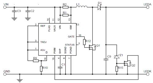
Figure 42: Application circuit - 400mA Boost LED driver
