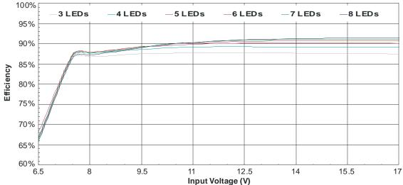
Figure 12: Efficiency vs. Input Voltage & Number of LED
