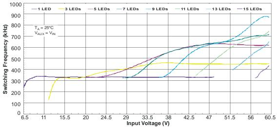
Figure 2: Frequency vs. Input Voltage & Number of LED
