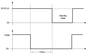
Fig 32: Stand-by state from PWM signal
