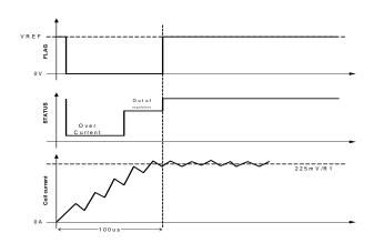
Fig 35: Diagnostic during Start-up
