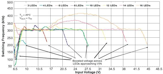
Figure 8: Frequency vs. Input Voltage & Number of LED
