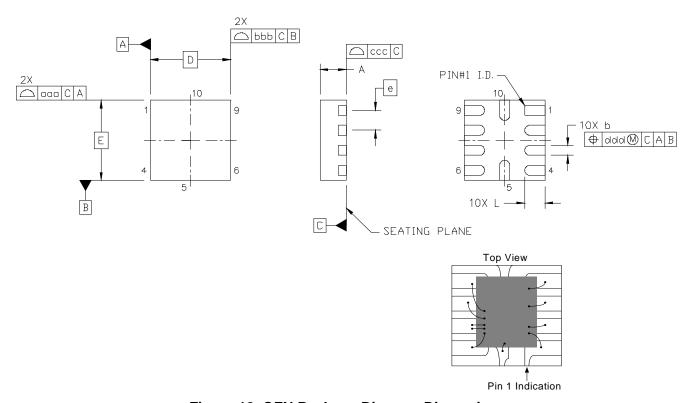
Figure 12. QFN Package Diagram Dimensions
