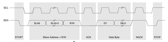
Figure 5. I<sup>2</sup>C Bit Timing Diagram
