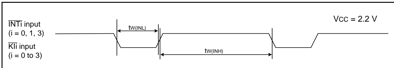
Figure 5.19 Input Timing for External Interrupt \overline{INTi} and Key Input Interrupt \overline{Kli} when Vcc = 2.2 V
