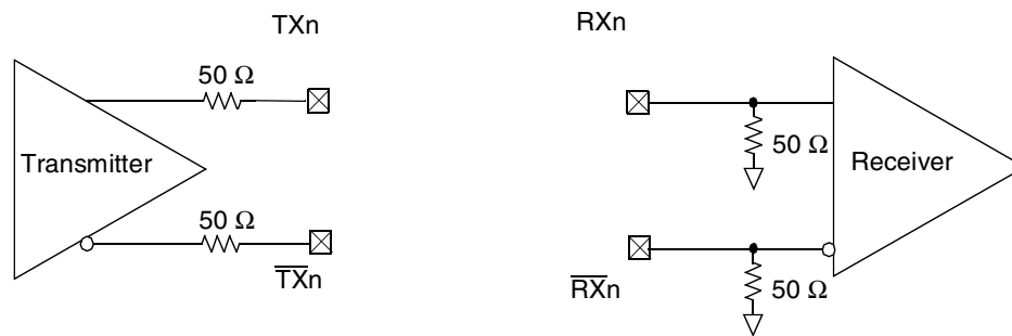
Figure 49. SerDes Transmitter and Receiver Reference Circuits
