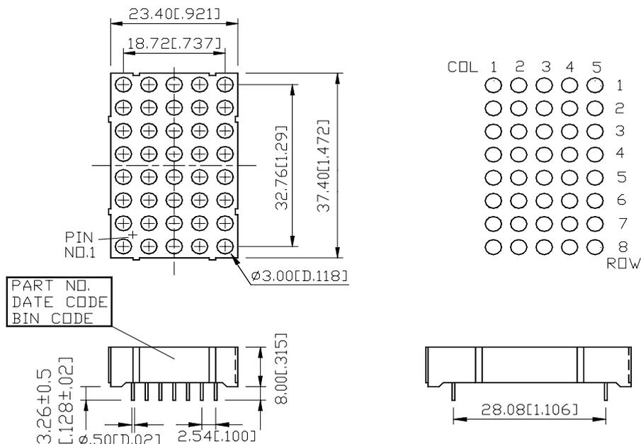
NOTES: All dimensions are in millimeters. Tolerance is  $\pm 0.25$  mm (0.01") unless otherwise noted.
