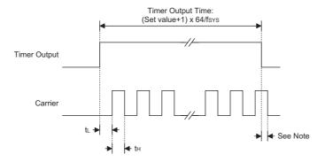
Timer Output when Carrier Is an Output
