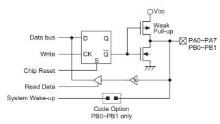
PA, PB0~PB1 Input/Output Lines
