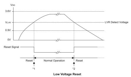
Note: "\*1" To make sure that the system oscillator has stabilised, the SST provides an extra delay of 1024 system clock pulses before entering normal operation.
