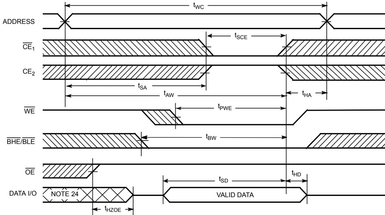
Figure 9 shows  $\overline{WE}$  controlled,  $\overline{OE}$  LOW write cycle waveforms.<sup>[23]</sup>
