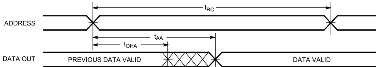
Figure 6 shows  $\overline{OE}$  controlled read cycle waveforms.<sup>[20, 21]</sup>
