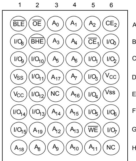
Figure 2. 48-Pin TSOP I Top View [3, 4]
