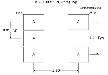
Figure 2. PCB Solder Mask (Top View)
