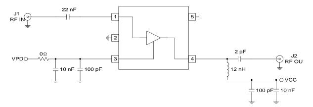
Application Schematic: Driver Amplifier ~1880MHz Operation
