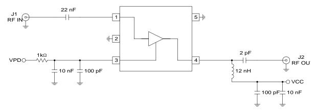
Application Schematic: Low Noise Amplifier ~1950MHz Operation
