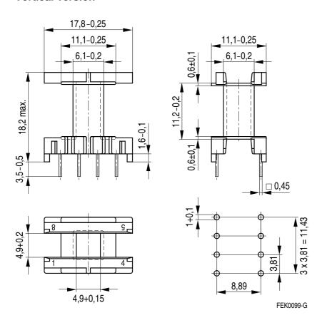
Hole arrangement View in mounting direction
