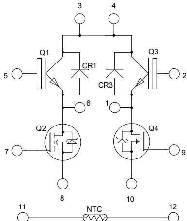
Top switches : Trench + Field Stop IGBT®
