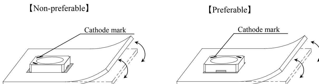
When mechanical stress from the board affects the soldered LED, place the LED in the preferable location and orientation as shown above.
