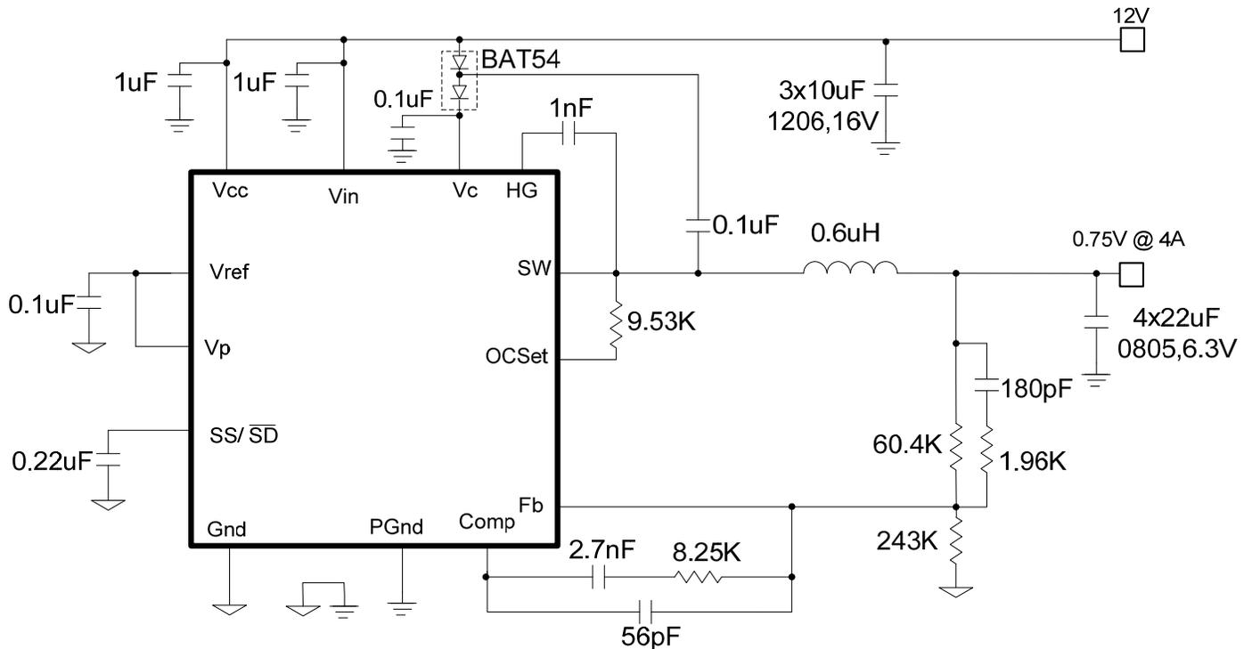
Fig.16: Typical Application circuit for 12V to 0.75V at 4A using ceramic output capacitors
