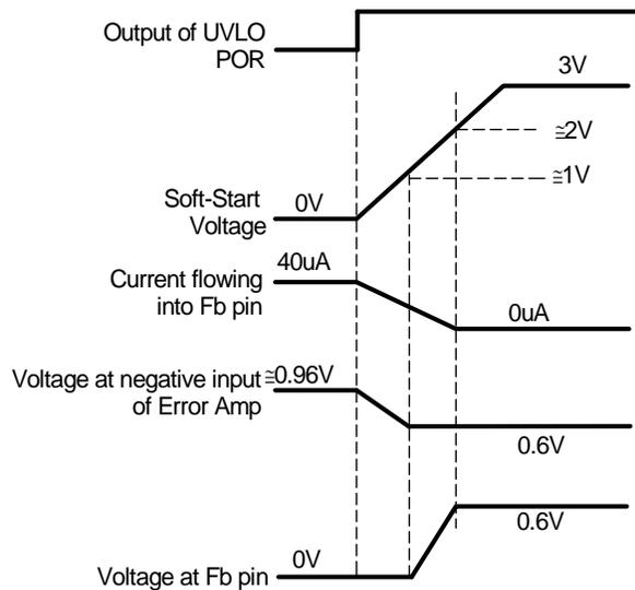
Fig. 6: Theoretical operation waveforms during soft-start
