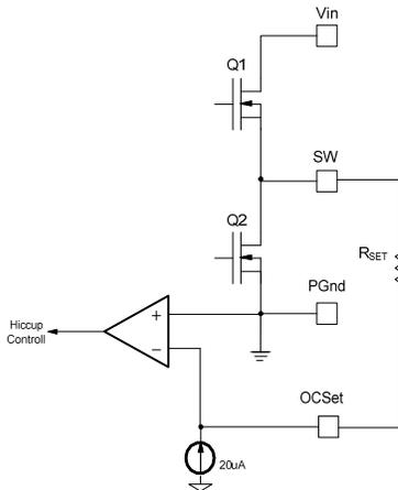
Fig. 7: Connection of over current sensing resistor
