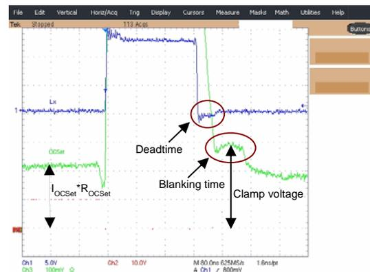
Fig. 9: OCset pin during normal condition
