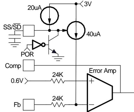
Fig. 5: Soft-Start circuit for IR3812
