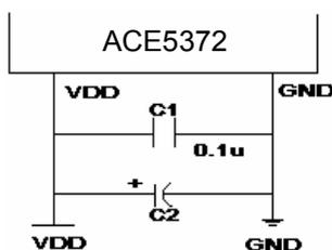
The VDD pin is connected to the positive power supply and GND to the ground. To prevent the possibility of noise, when rapidly changing signal took place on ACE5372 pin, we have to place a capacitance beside the ACE5372. One possibility is to place a bypass capacitance as close as to the ACE5372. The capacitance capacity of C2 could be determined per user's demand, which provides large current passing ability between the pin and the ground.
