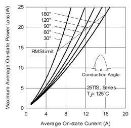
Fig. 3 - On-State Power Loss Characteristics
