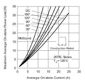
Fig. 4 - On-State Power Loss Characteristics
