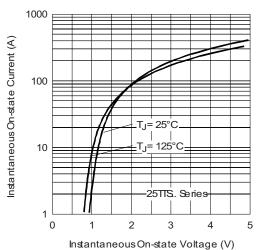
Fig. 7 - On-State Voltage Drop Characteristics
