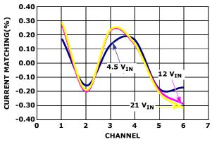
FIGURE 8. CHANNEL-TO-CHANNEL CURRENT MATCHING
