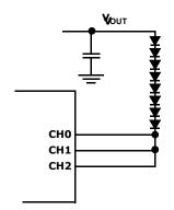
FIGURE 40. GROUPING MULTIPLE CHANNELS FOR HIGH CURRENT APPLICATIONS
