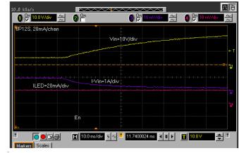
FIGURE 14. LINE REGULATION WITH V<sub>IN</sub> CHANGE FROM 6V TO 26V, V<sub>IN</sub> = 12V, 6P12S AT 20mA/CHANNEL
