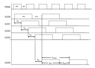
FIGURE 22. PHASE SHIFT WITH FIXED DELAY (4 CHANNELS)
