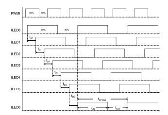
FIGURE 21. PHASE SHIFT WITH FIXED DELAY (6 CHANNELS)
