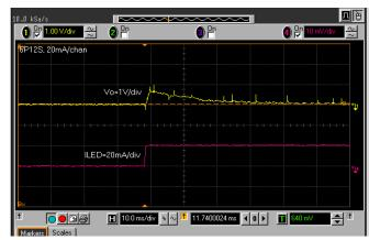
FIGURE 16. LOAD REGULATION WITH I<sub>LED</sub> CHANGE FROM 0% TO 100% PWM DIMMING,  $V_{IN}$  = 12V, 6P12S AT 20mA/CHANNEL
