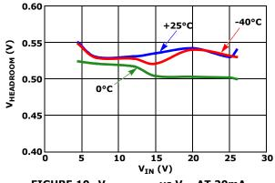
FIGURE 10.  $V_{HEADROOM}$  vs  $V_{IN}$  AT 20mA
