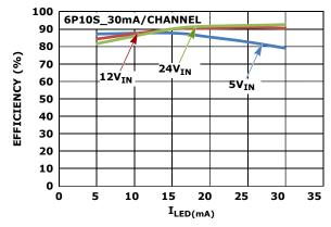
FIGURE 4. EFFICIENCY vs up to 30mA LED CURRENT (100% LED DUTY CYCLE) vs V<sub>IN</sub>
