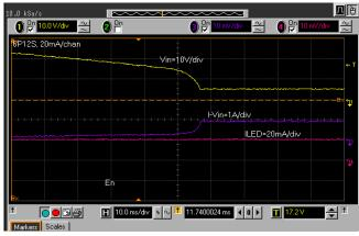
FIGURE 15. LINE REGULATION WITH V<sub>IN</sub> CHANGE FROM 26V TO 6V FOR 6P12S AT 20mA/CHANNEL
