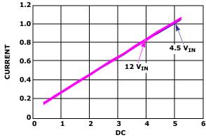
FIGURE 9. CURRENT LINEARITY vs LOW LEVEL PWM DIMMING DUTY CYCLE vs V<sub>IN</sub>
