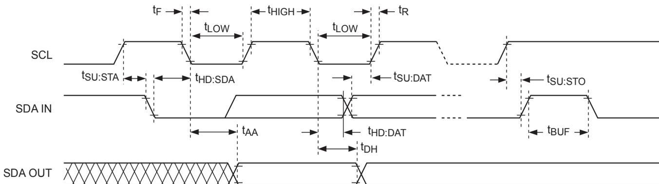
**Figure 1. I<sup>2</sup>C Bus Timing Characteristics**
