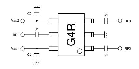
Off chip DC blocking capacitors value C1 = 56 pF, C2 = 1 000 pF (Bypass), using NEC standard evaluation board.
