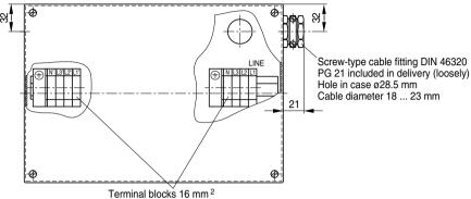
Tightening torque 1.5 ... 1.8 Nm
