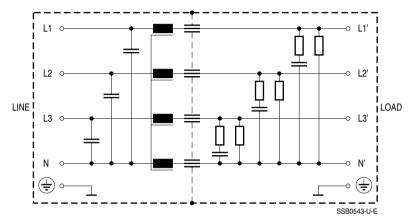
Typical circuit taking the example of filters for 16 A
