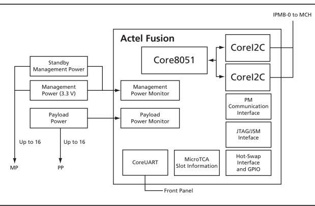
Figure 2 • Power Module Fusion Device Block Diagram
