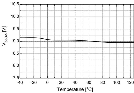
Figure 7. V<sub>DD</sub> UVLO- vs. Temperature
