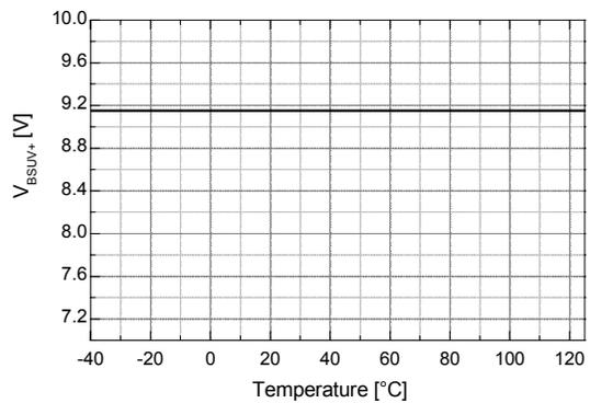
Figure 8. V<sub>B</sub>.V<sub>OUT</sub> UVLO+ vs. Temperature
