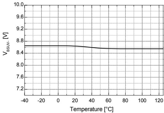
Figure 9. V<sub>B</sub>.V<sub>OUT</sub> UVLO- vs. Temperature
