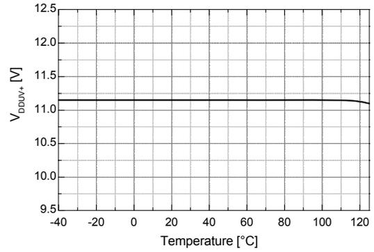
Figure 6. V<sub>DD</sub> UVLO+ vs. Temperature
