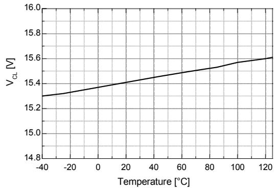
Figure 10. V<sub>CL</sub> vs. Temperature
