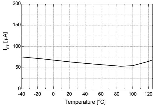
Figure 5. Startup Current vs. Temperature
