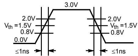
TTL Input Test Waveform (CY7B9911)
