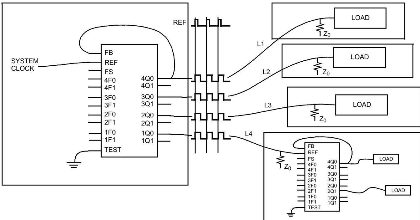
Figure 8 shows the CY7B9911 connected in series to construct a zero-skew clock distribution tree between boards. Delays of the downstream clock buffers are programmed to compensate for the wire length (that is, select negative skew equal to the wire delay) necessary to connect them to the master clock source,
