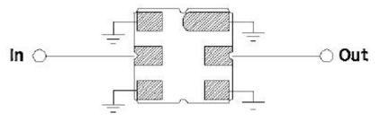
Load/ Source Impedance = 50 ohms
