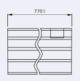
Tube for THT version 50 relays per stick 1'000 relays per box
