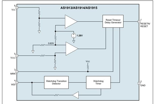
Figure 9. Functional Diagram of Vcc Supervisory Application
