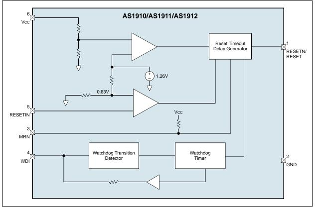
Figure 11. Functional Diagram of RESETIN Supervisory Application
