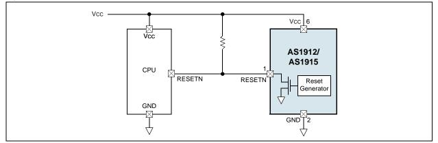
Figure 14. AS1912 or AS1915 RESETN-to-CPU Bi-Directional Reset Pin
