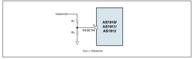
To monitor a voltage higher than 0.63V, connect a resistor divider network to the circuit as shown in Figure 12. For the circuit shown in Figure 12, the threshold at VMONITOR is:
