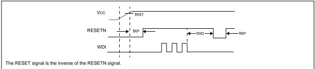
The watchdog is internally driven low during most (87.5%) of the watchdog timeout period (see two on page 6) and high for the rest of the watchdog timeout period. When pin WDI is left unconnected, this internal driver clears the watchdog timer every 1.4s. When WDI is tri-stated or is not connected, the maximum allowable leakage current is 10µA and the maximum allowable load capacitance is 200pF.
