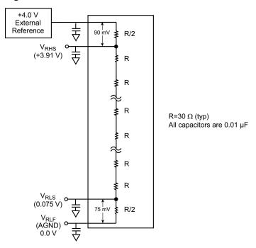
(chip cap preferred) to minimize high-frequency noise injection. If this simplified configuration is used, the following considerations should be taken into account.
