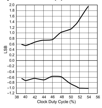
Figure 8 - ILE vs Clock Duty Cycle
