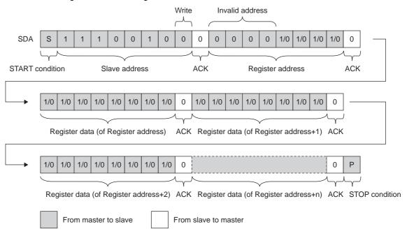
Continuous data transmission after transmission of initially-set address data of register • data writing sequence enables writing of data in the consecutive register • data area. In this case, the register • address increases by one address from the initially-set address of the sequence and continues increasing till the "Stop" condition (P) is generated.
