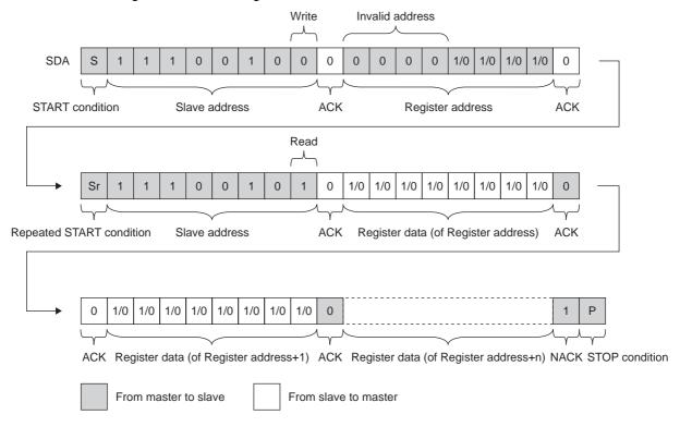
When the master returns ACK (0 data) after reading of the initial register • address • data of read sequence, the register • address increases by one address, enabling consecutive reading of data corresponding to each register address. If the master does not return ACK (0 data), the register address does not increase.
