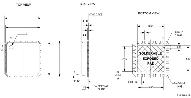
Figure 18. 32-Pin QFN (5 x 5 mm)
