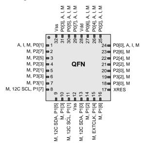
Figure 7. CY7C60333-LFXC 32-Pin Device
