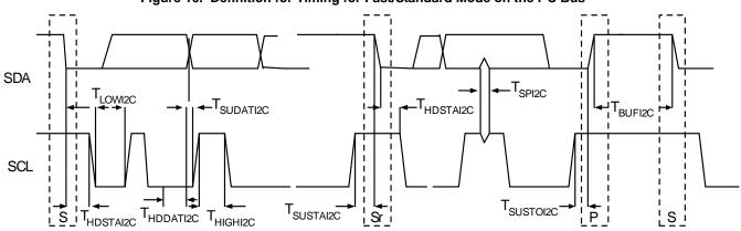
Figure 16. Definition for Timing for Fast/Standard Mode on the I<sup>2</sup>C Bus
