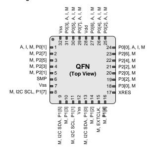
Figure 9. CY7C60333-LTXC 32-Pin Device
