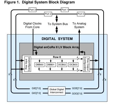
The digital blocks may be connected to any GPIO through a series of global buses that can route any signal to any pin. The buses also allow for signal multiplexing and for performing logic operations. This configurability frees your designs from the constraints of a fixed peripheral controller.
