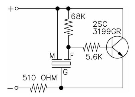
The current consumption and the sound pressure level are measured by using the recommended driving circuit shown above.
