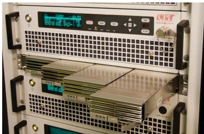
SSPA with optional redundant hot-swappable power supplies
