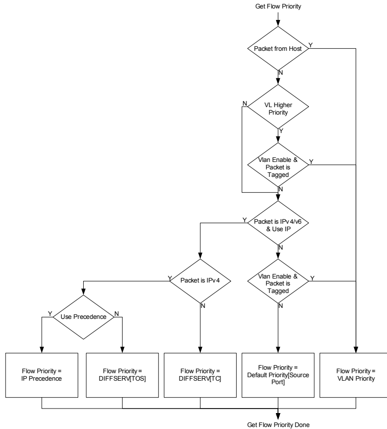
Figure 6.8 Switch Engine Ingress Flow Priority Calculation
