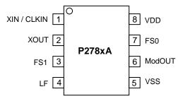
Standard pin Configuration offered in both 8 pin SOIC Packages.
