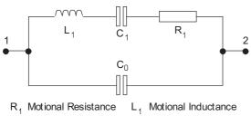
C1 Motional Capacitance C0 Shunt Capacitance
