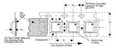
Figure 6. Tape and Reel Mechanical Data
