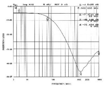
Figure 3. Microphone Circuit (A5-C5) EMI Filter Performance
