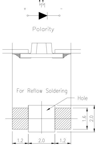
**Note:** The tolerances unless mentioned is  $\pm 0.1$ mm ,Unit = mm
