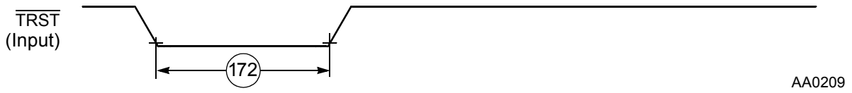
Figure 36. \overline{\text{TRST}} Timing Diagram
