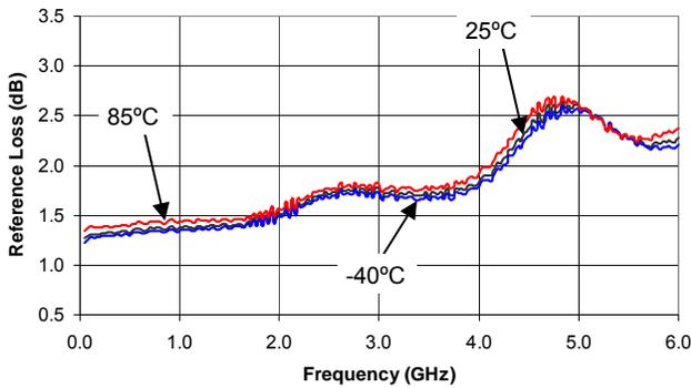
Attenuation - 16 dB Bit (C1) vs. Frequency
