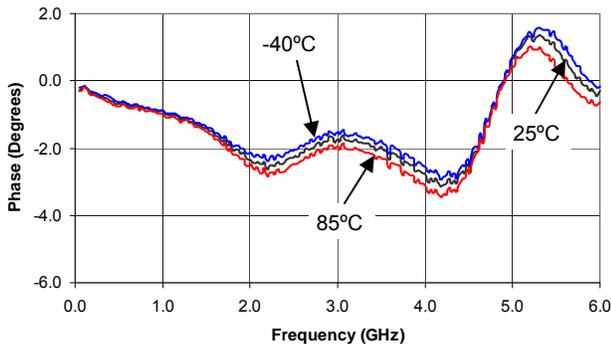
Phase - 16 dB Bit (C2) vs. Frequency
