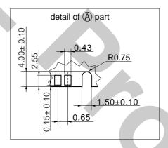
Note: The dimensions without tolerance specification use the default tolerance of  $\pm$  0.13.
